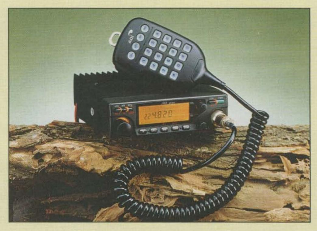
Front panel of ADI's AR-247 mobile rig for 222–225 MHz. The controls are easy to access, even without looking at the radio, and the big LCD display makes for easy viewing when you do look at it. (Photo courtesy of ADI.)
