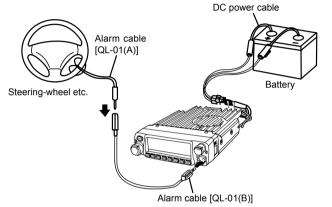
Connect DC power cable with car battery.
