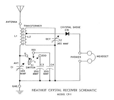
The Heath CR-1 measures 6" x 3" x 2" wide. The case is bakelite with a gray-metal top plate that is the front panel. Similar cases are available today at a lot of stores including Radio Shack. The circuit, shown in Figure 1, is a double tuned circuit followed by the crystal detector circuit that feeds the headphones.
