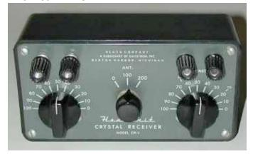
Over a period of about five years (1957 - 1962) Heathkit also sold a crystal radio set kit, the CR-1. This radio, like most, tuned the AM broadcast band from 540 KHz to 1600 KHz (kc in those days). The CR-1 is a simple kit that uses a sealed crystal diode instead of a "cats-whisker". It is double tuned and drives high impedance headphones. It is a cherished Heathkit among collectors. However you can build your own for a lot less than the kit seems to be going for on eBay.
