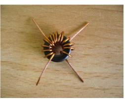
Important: Wind the toroid exactly as shown in the pictures. You must respect both the number of turns as the winding direction.
