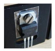
The Q7 encapsulation must be electrically isolated from the radiator. Use talked washer and mica sheet that came with the transistor. Once clamped transistor, check with a multimeter that the transistor housing does not contact the screw or the radiator. Use the insulators supplied with a screw and a nut M3.It is advisable to apply some thermal paste.
