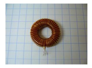
L6 can be wound in two stages. Spend half of the wire through the toroid, wind around the half of the toroid, then, rotate the toroid and wind to complete the other half. If you are unsure of how many turns given. With a magnifying glass and focus can easily count.
