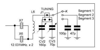
The capacitors must be of good quality such as "NPO" "Styroflex" or similar to avoid adversely affected the stability of the VXO.
