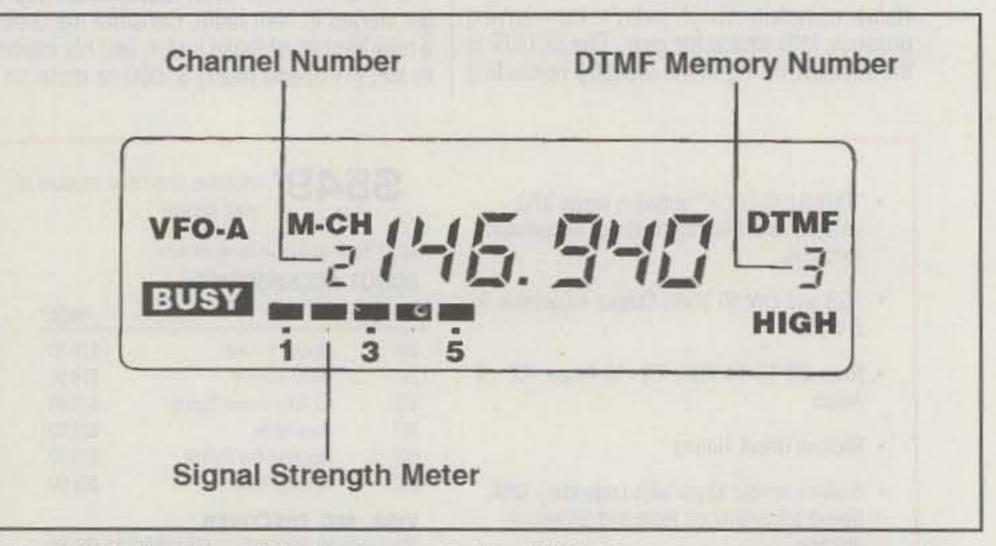
Fig. 1– This illustration of the display panel of the HTX-212 two meter transceiver was taken from the instruction manual.
