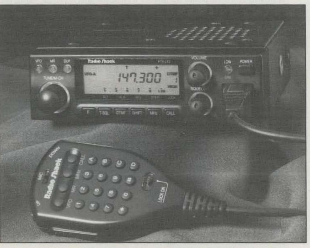
Subaudible tones for transmit and receive are also included for closed systems.
