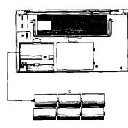
Insert the bottom projections on the edge of the battery compartment cover inside the lower edge of the compartment opening. Lower the cover, and snap the top latch down until it clicks closed.
