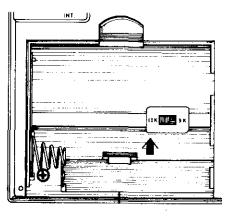
3. Insert six D batteries in the main battery compartment. Position them as shown in the illustration on the back of the radio. For best results, use alkaline batteries such as Radio Shack<sup>®</sup> Cat. No. 23-550.
