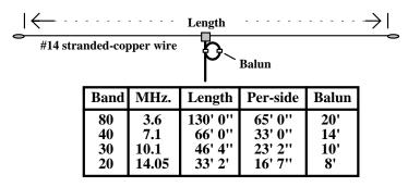
Balun consists of RG58 coiled 10" in diameter and held with tape or plastic tie-wraps
