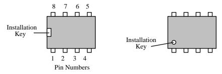
□ □ 46. Align the NE602 so the installation key corresponds with markings on the pc board at U1. Carefully insert the pins into the mounting holes provided, seating the device firmly in place. Confirm all pins protrude through the board, and that none were bent over during insertion. The keyed end should be positioned toward the front of the pc board.
