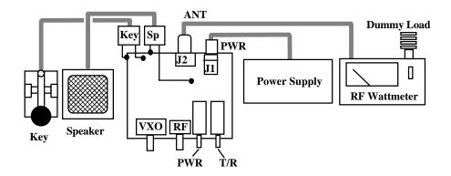
To test the radio outside of a metal case, you'll need to install temporary "ground" or "common" leads for the key and speaker jacks. Use temporary lenghts of hookup wire or clipleads to make these connections. These may be attached to any convenient point on the pc board ground surface.
