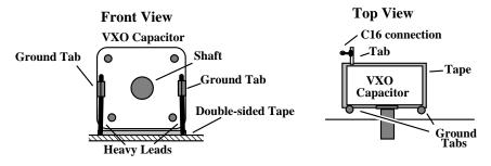
□ 10. Install two (2) heavy leads (from the 1N4007 diode) from the ground tabs to the pads provided on the front of the pc board. Solder each lead at both ends. The combined holding action of the two-sided tape and the ground leads should anchor the cap firmly in place. Rotate the cap through its range--the capacitor should not shift position.
