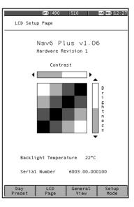
If 'Night Preset' is visible in the softkey menu area then the contrast and brightness control bars show the current 'Night' settings. These can be changed using the LEFT, RIGHT, UP and DOWN keys.
