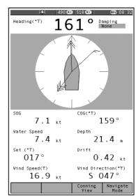
The Conning Display is a unique analogue display which shows overlapping vectors for Heading (course through the water), Course Over the Ground (COG), Set (a combination of leeway and tide) and wind. All these vectors are displayed relative to the current heading, which is displayed in digital form at the top of the screen.
