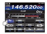
Touch [GROUP] on the LCD, then rotate the MULTI knob, or touch the screen to select the station that you would like to register.
