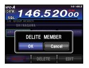
5. Touch [**DELETE**] on the LCD. A deletion confirmation screen will be displayed.
