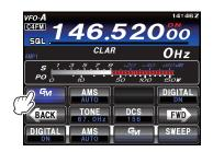
Up to 24 stations operating with the GM function within the sphere of communications will be listed on the TFT display.
