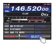
4. Touch [ENTER] on the LCD, then touch [BACK] on the LCD or press the **MENU** button to save the new setting and exit to normal operation.
