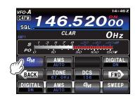
Touch [GROUP] on the LCD, then rotate the MULTI knob, or touch the screen to select a new box with "NEW" displayed on the left hand side.
