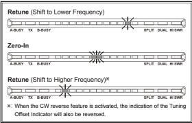
O The LED Bar Display can be utilized for a graphical representation of the operation of the CW-TUNE, Clarifier, VRF/μ-TUNE, or IF Notch function. Use Menu [DISPLAY 016 BAR DISPLAY SELECT] to engage the desired display function.
