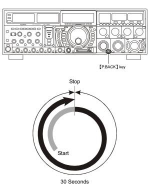
The **[**P/B**]** key of the supplied FH-2 Keypad can also serve as a remote-control recording/playback switch. Operation is described below.
