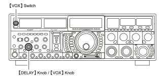
**[Advice]** VOX operation may be engaged on either Voice modes (SSB/AM/FM) and on AFSK-based Data modes. Use Menu item [TX GNRL 159 VOX SELECT] (the selections are "MIC" and "DATA").
