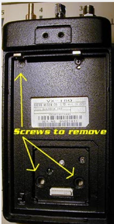
Fig 2 Remove screws
