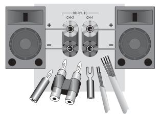
Figure 3.5 Output Connector Wiring
