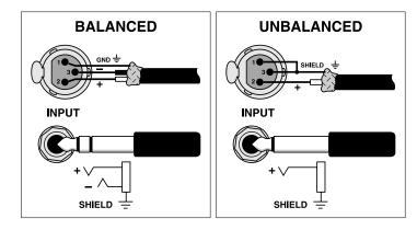
Figure 3.3 Balanced Input Connector Wiring Figure 3.4 Unbalanced Input Connector Wiring
