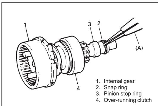
7) Remove snap ring, then pull out pinion stop ring and over-running clutch and internal gear.
