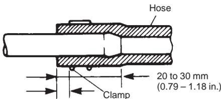
Clamp securely at a position 3 to 7 mm (0.12 - 0.27 in.) from hose end.
