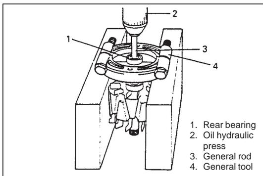
7) When removing rear bearing, use oil hydraulic press.
