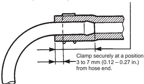
With straight pipe, fit hose till pipe is about 20 to 30 mm (0.79 - 1.18 in.) into the hose.
