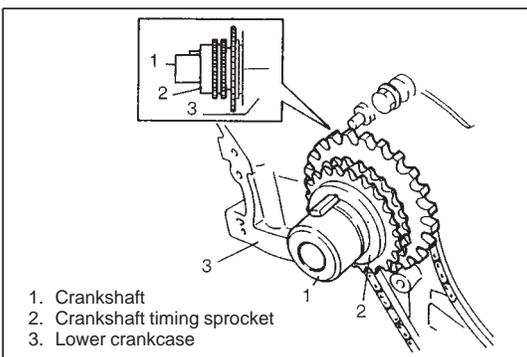
2) Install 1st timing chain crankshaft sprocket as shown in figure. Confirm that tooth for CKP sensor are free from metal particles and damage.
