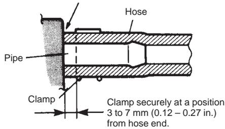
With following type pipe, fit hose as far as its peripheral projection as shown.
