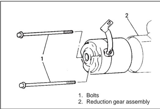
2) Remove bolts shown in left figure, then separate reduction gear assembly from starting motor assembly.
