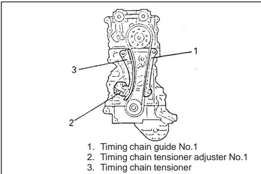
9) Remove timing chain guide No.1.
