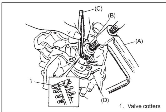
8) Using special tool (Valve lifter), compress valve spring and fit two valve cotter pins into groove in valve stem.
