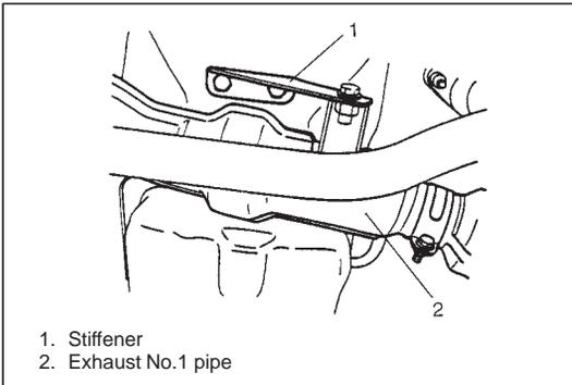
11) Detach exhaust manifold stiffener from transmission case.
