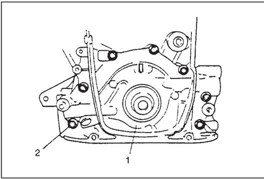
6) Remove oil pump assembly (1) after removing bolts (2).
