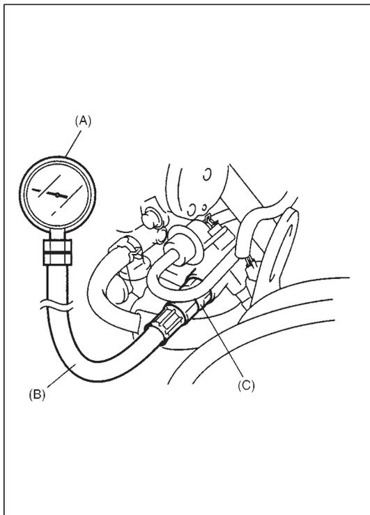
2) Using backup wrench, loosen plug bolt on fuel delivery pipe and remove it. Connect special tools (fuel pressure gauge) to delivery pipe.
