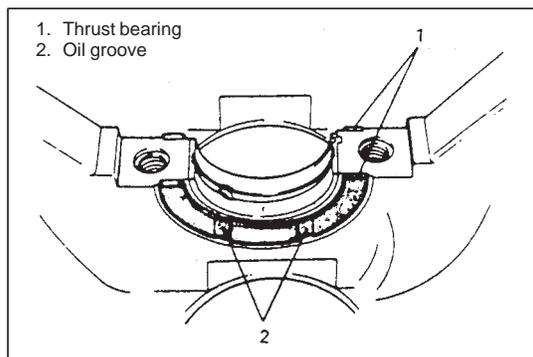
2) Install thrust bearings to cylinder block between No.2 and No.3 cylinders. Face oil groove sides to crank webs.
