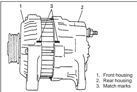
1) For easier reinstallation, provide match marks on both front and rear housings as shown in left figure before separating them.
