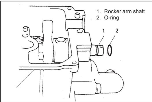
13) Push off rocker arm shaft end to CMP sensor case side and remove O-ring from shaft.
