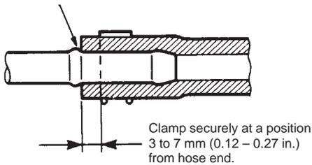
With bent pipe, fit hose as far as its bent part as shown or till pipe is about 20 to 30 mm (0.79 - 1.18 in.) into the hose.
