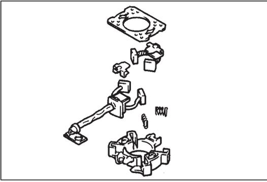
12) Remove rear bracket cap, and then remove rear bush, as required.
