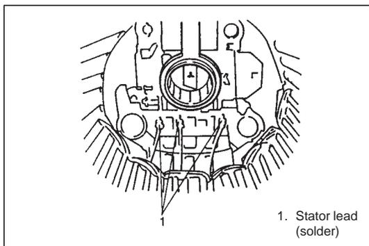
9) Unsolder stator leads and remove stator from rear housing and regulator assembly.
