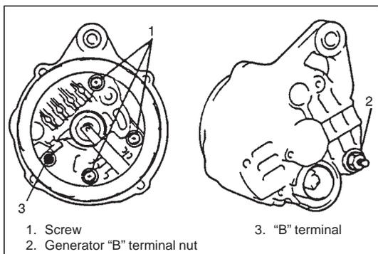
8) Remove three screws and generator "B" terminal nut.
