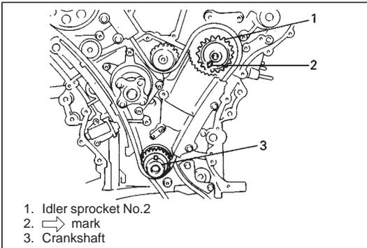
2) Check timing mark on idler sprocket No.2 as shown in figure.
