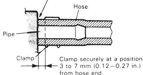
With following type pipe, fit hose as far as its peripheral projection as shown.
