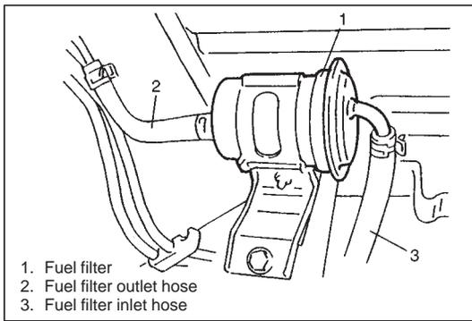
8) Disconnect fuel filter inlet hose from filter.
