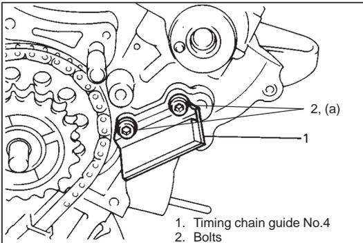
3) Install timing chain guide No.4.
