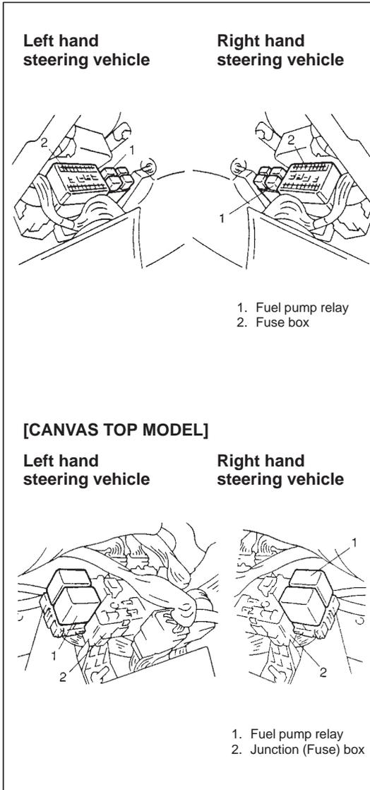
**FUEL LEAKAGE CHECK PROCEDURE**
