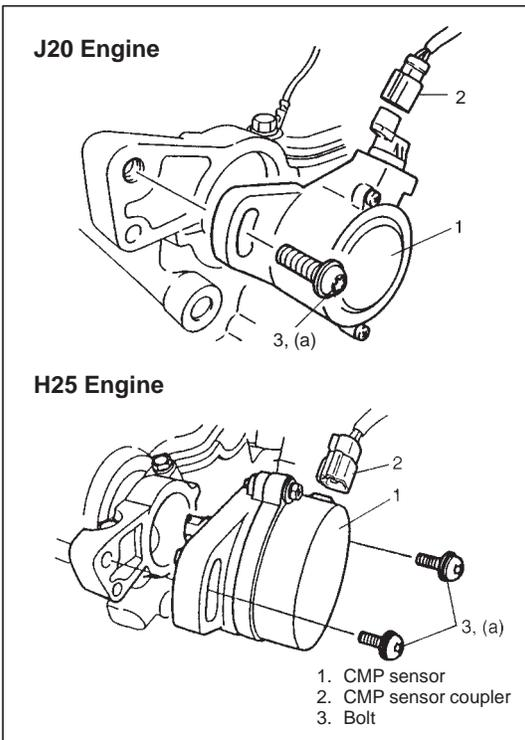
3) Tighten CMP sensor bolts.
