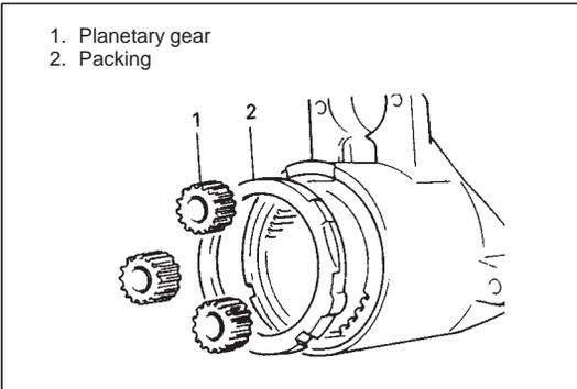
3) To overhaul reduction gear assembly, remove packing and planetary gears.
