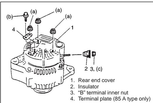
16) Install insulator and tighten "B" terminal inner nut to specified torque.
