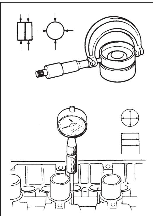
Measure cylinder head bore and adjuster outside diameter to determine cylinder head-to-adjuster clearance. If clearance exceeds limit, replace adjuster or cylinder head.
