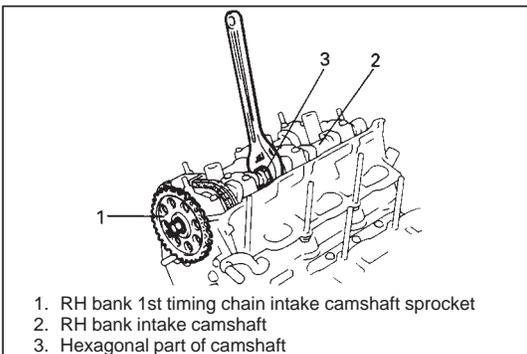
1. RH bank 1st timing chain intake camshaft sprocket
