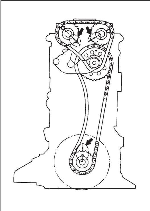
7) For reinstallation of timing chain, turn crankshaft so that timing marks on cylinder head and cylinder block match with those on sprockets as shown in figure.
