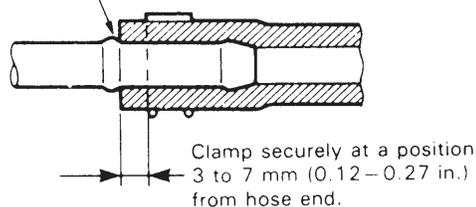
With bent pipe, fit hose as far as its bent part as shown or till pipe is about 20–30 mm (0.79–1.18 in.) into hose.
