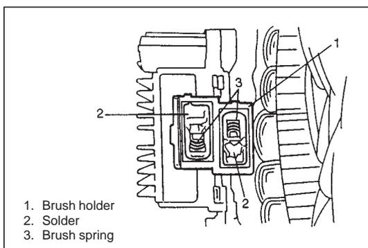
10) To remove brush, remove holder cover from brush holder and then disconnect brush wire from regulator terminal by using soldering iron.
