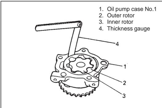
° Measure clearance of oil pump rotor and oil pump case.
