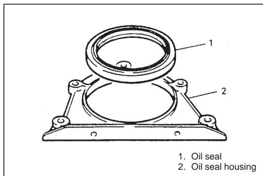
For oil seal installation, press-fit rear oil seal so that oil seal housing end face is flush with oil seal end face.
