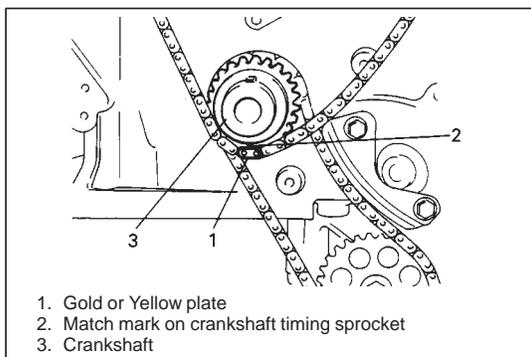
10) Install crankshaft sprocket by aligning match marks on gold or yellow plate of 1st timing chain and crankshaft timing sprocket. To install it, fit a spanner to hexagonal part at the center of RH bank intake camshaft to turn a little.
