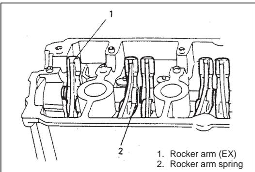
14) Remove exhaust rocker arms and rocker arm spring by pulling rocker arm shaft to front side.
