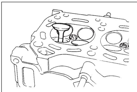
6) Install valve to valve guide.
