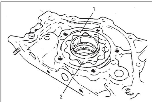
3) Remove outer rotor (1) and inner rotor (2).
