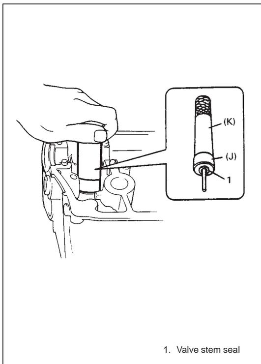
5) Install new valve stem seal to valve guide.
