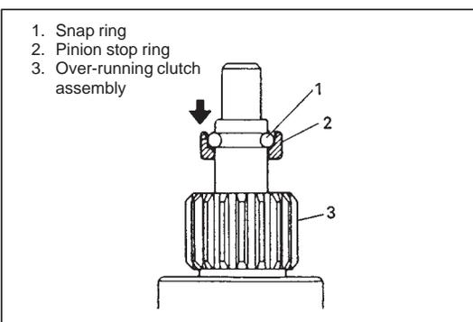
6) Loosen pinion stop ring fixed by snap ring.
