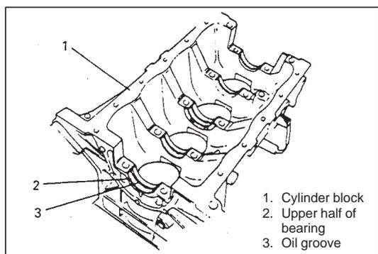
1) Install main bearings to cylinder block.
