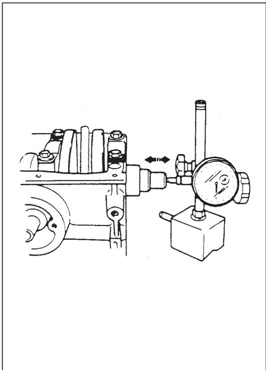
Use a dial gauge to read displacement in axial (thrust) direction of crankshaft.
