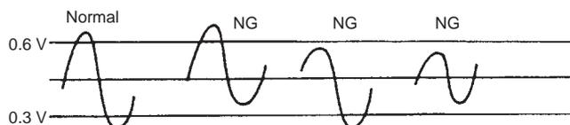
**DTC P0133 HO2S-1 CIRCUIT SLOW RESPONSE****WIRING DIAGRAM**
