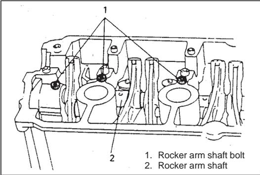
12) Remove rocker arm shaft bolts.
