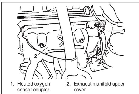
1. Heated oxygen sensor coupler
