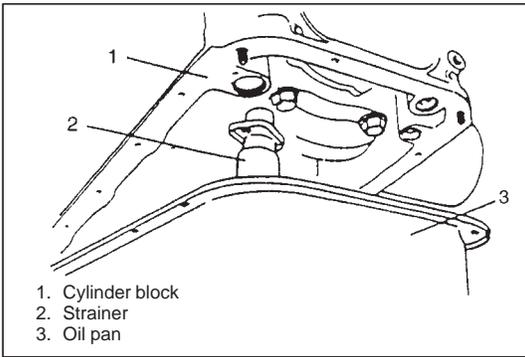
6) Remove oil pan and then oil pump strainer.
