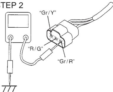
**DTC P0121 THROTTLE POSITION CIRCUIT PERFORMANCE PROBLEM****WIRING DIAGRAM**
