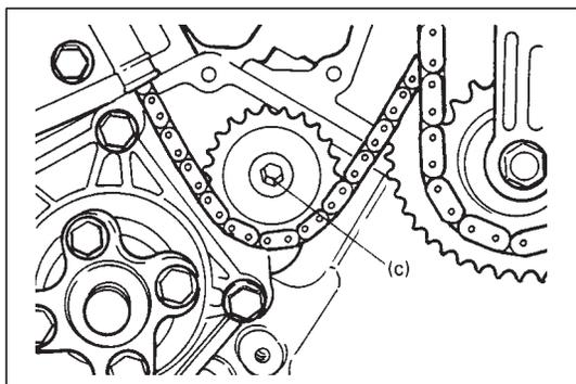
11) Apply oil to bearing of idler sprocket No.1.
