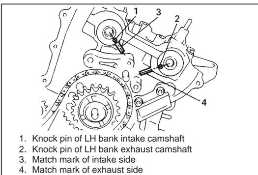
4) Check that knock-pins of intake and exhaust camshafts are aligned with match marks on cylinder head as shown in figure.
