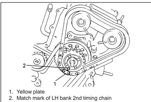
5) Install by aligning match marks on yellow plate of LH bank 2nd timing chain and idler sprocket No.2.
