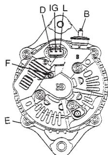
B : Generator output (Battery terminal)
