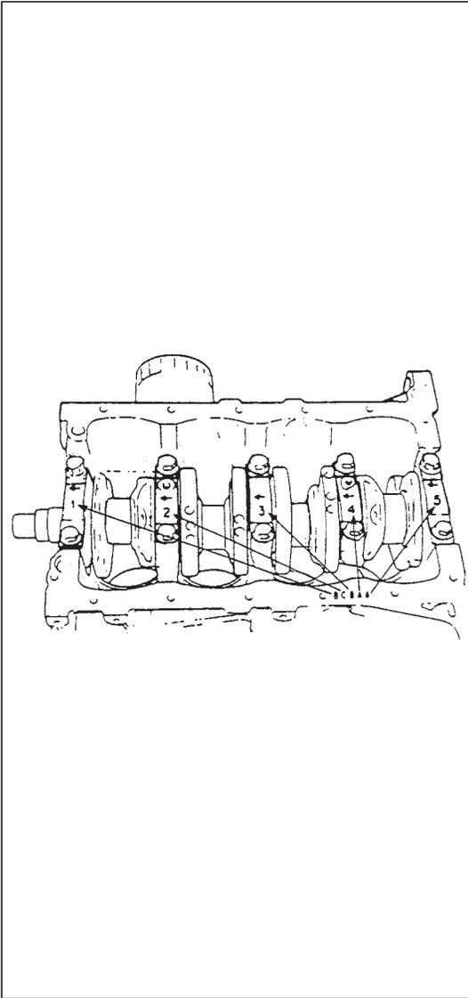
2) Next, check bearing cap bore diameter without bearing. On mating surface of cylinder block, four alphabets are stamped as shown in figure.
