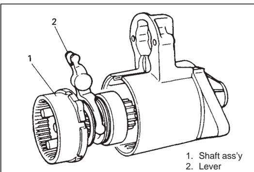
5) Remove shaft assembly with lever.
