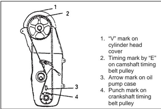
8) Remove timing belt tensioner, tensioner plate, tensioner spring and timing belt.
