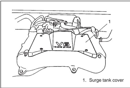
7) Remove air cleaner upper case, intake air hose, intake air pipe and surge tank pipe as one component. Do not disassemble them, when removing and reinstalling.
