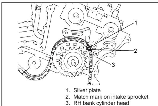
9) Install idler sprocket No.2 by aligning match marks on LH silver plate of 1st timing chain.
