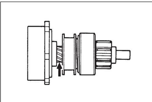
◦ Inspect spline teeth for wear or damage. Replace if necessary. Inspect pinion for smooth movement.
