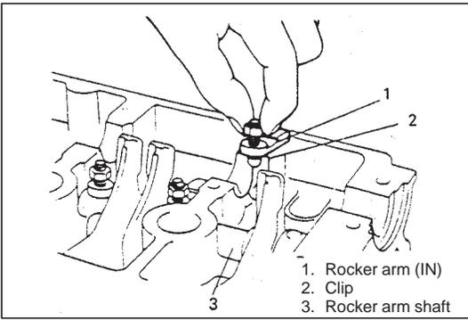
11) Remove intake rocker arm with clip from rocker arm shaft.
