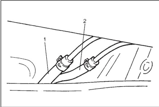
9) Disconnect fuel vapor hose (1) and return hose (2) from pipes.
