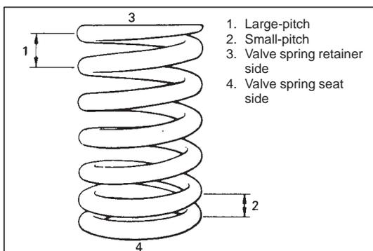
7) Install valve springs (inner and outer) and spring retainer.
