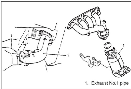
13) Disconnect exhaust No. 1 pipe from exhaust manifold.
