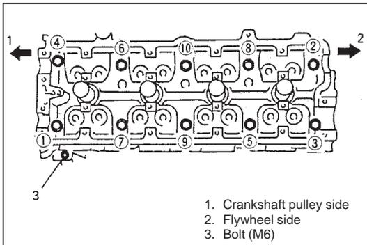
15) Loosen cylinder head bolts in such order as indicated in figure and remove them.
