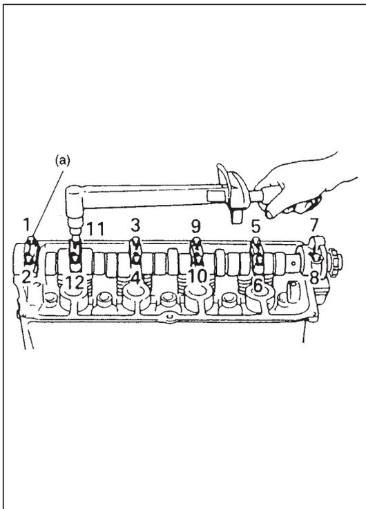
Check clearance by using gaging plastic.
