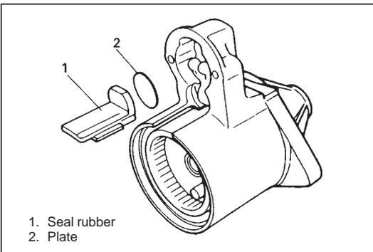
4) Remove seal rubber and plate.
