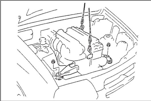
24) Install lifting device.
