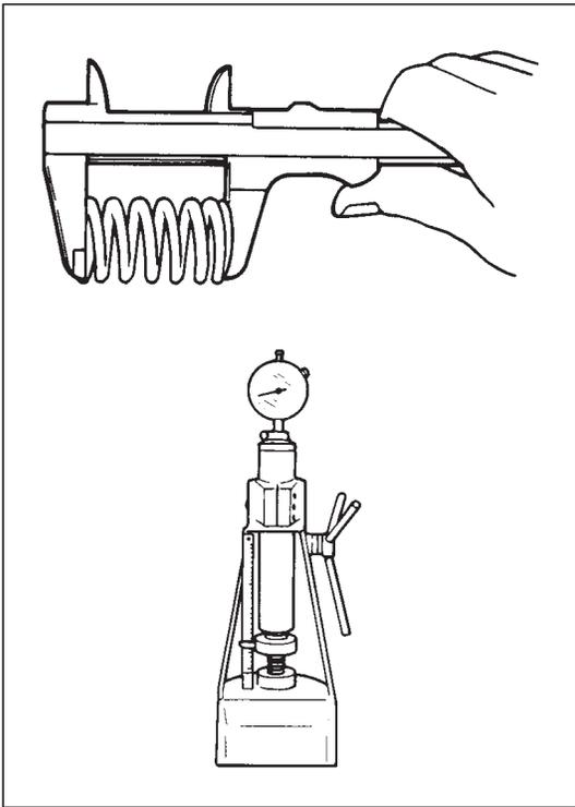
° Measure free length and tension of oil relief spring.
