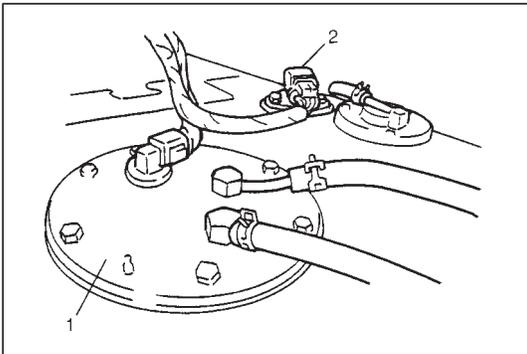
11) Lower fuel tank gradually while holding it horizontally and pull out each coupler from fuel pump (1) and fuel tank pressure sensor (2).
