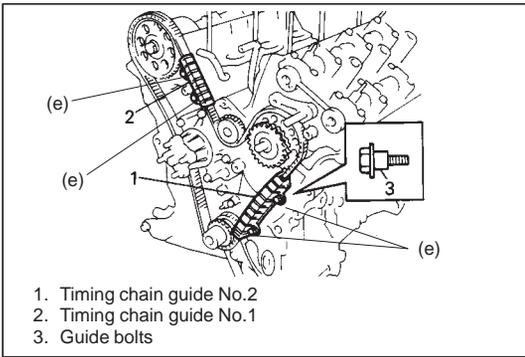
17) Check each aligned timing marks as shown in figure.
