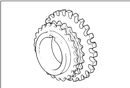
**RH bank 1st timing chain intake camshaft sprocket**
