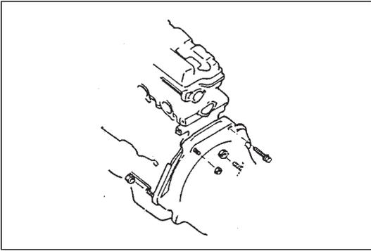
23) Remove bolt and nuts fastening cylinder block and transmission.
