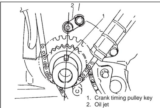
1. Crank timing pulley key
