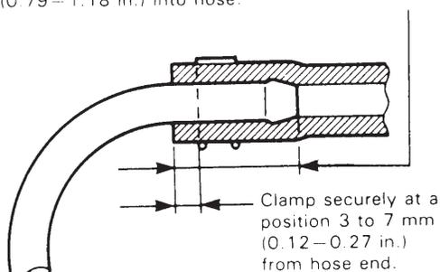
With straight pipe, fit hose till pipe is about 20 to 30 mm (0.79–1.18 in.) the hose.
