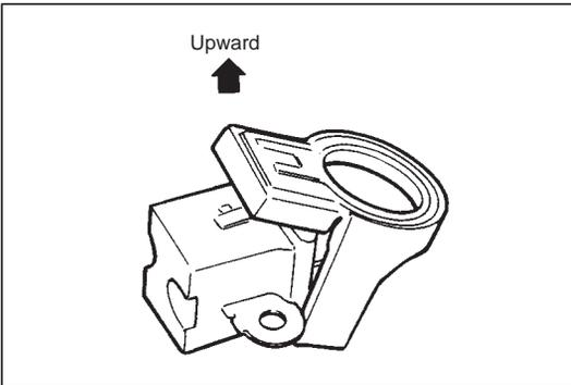
13) Place the IC regulator together with the brush holder horizontally on the rear end frame.
