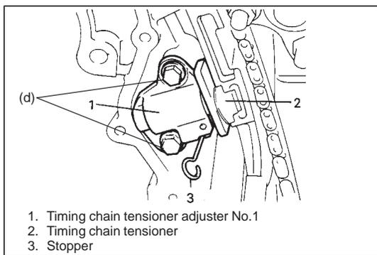
14) Install timing chain tensioner adjuster No.1.
