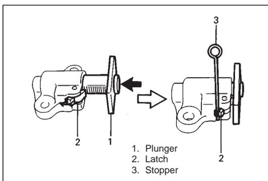
13) With latch of tensioner adjuster No.1 returned and plunger pushed back into body, insert stopper into latch and body. After inserting it, check to make sure that plunger will not come out.
