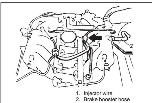
12) Disconnect couplers of TP sensor, MAF sensor and IAC valve.
