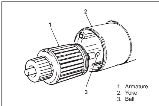
9) Remove armature from yoke and then ball from the end of armature shaft.
