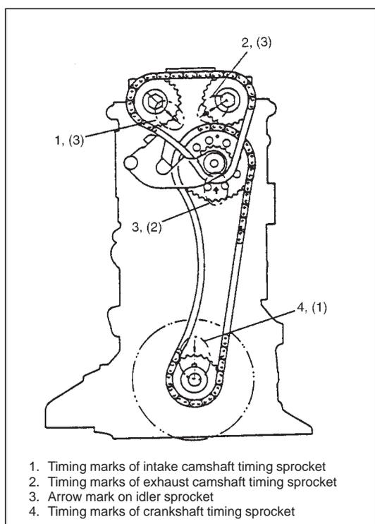
1. Timing marks of intake camshaft timing sprocket
