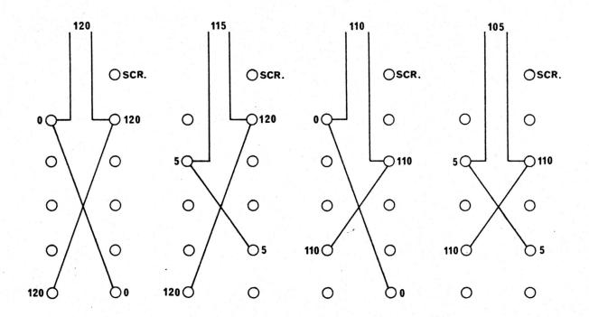
FIGURE 1 - TRANSFORMER PRIMARY CONNECTIONS.
