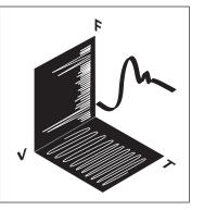
For timing measurements, the Modulation Domain's view of time interval vs. time allows you to both see and quantify timing jitter directly-taking you one step beyond the Time Domain's qualitative view.
