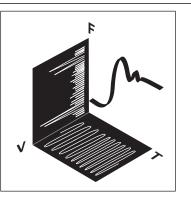
For timing measurements, the Modulation Domain's view of time interval vs. time allows you to both see and quantify timing jitter directly—taking you one step beyond the Time Domain's qualitative view. By internet, phone, or fax, get assistance with all your test and measurement needs.
