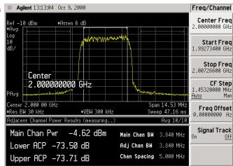
The usable dynamic range of the PSA is enhanced by a standard 2 dB step attenuator that covers the complete frequency range of the analyzer, and by the ability to switch off ADC dither to lower displayed-average noise level (DANL).
