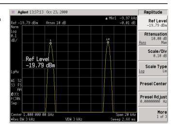
Accurate amplitude measurements challenge the entire analysis chain, including the input section, downconversion, signal processing, and detection.
