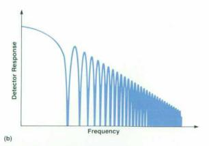
Fig. 10. Integrating detector measurement system characteristics. (a) Damped oscillation output of amplifier. (b) Response of integrating analog-to-digital detector versus frequency.
