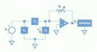
Fig. 1. Standard analog in-circuit measurement configuration for unknown component  $Z_x$ .
