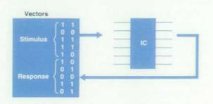
Fig. 1. Digital in-circuit testing is defined by vectors that describe the input test pattern and the expected response pattern for a device.
