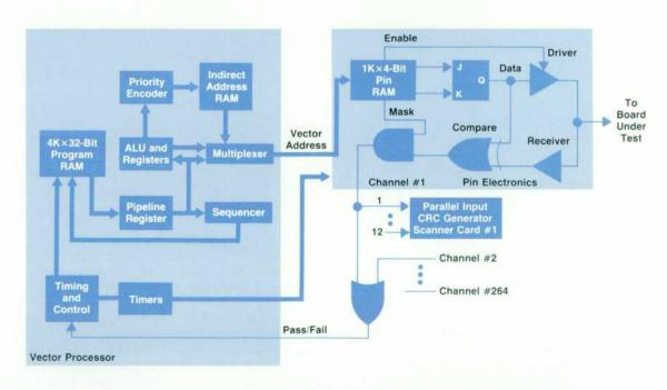
Fig. 2. Digital subsystem architecture of the HP 3065H Test Station (see Fig. 1) Although only the pin electronics block diagram for one test channel is shown, there are 12 channels on each digital scanner card and the HP 3065H can accommodate up to 22 cards or 264 channels.
