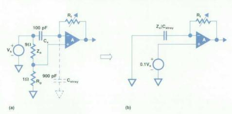
Fig. 7. The stray capacitance in the test system combined with the guard lead impedance as shown in (a) can be modeled by the circuit shown in (b) to calculate its effect on the measurement of Z<sub>x</sub>.
