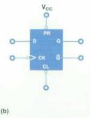
Fig. 5. (a) D-type flip-flop and library test sequence. (b) Use of flip-flop on board under test. For this topology, the library test is modified by removing test vector unit one.
