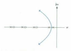
**Fig. 9.** The HP 3065 Board Test System compensates for part of the settling delay problem by introducing pole-zero pairs to the plot shown in Fig. 8c. This forms a locus of an approximately constant damping factor.
