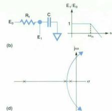
Fig. 8. A single-pole amplifier (a) and a single-pole input network (b) results in a closed-loop root-locus plot as shown in (c). By moving the network to the feedback path of the amplifier, another pole is introduced as shown in (d), causing longer settling delays or, in some cases, instability.
