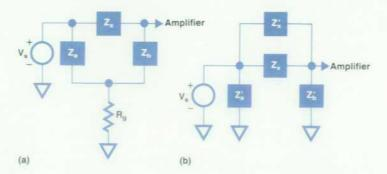
Fig. 6. The wye network (a) containing the guard lead impedance  $R_g$  can be converted to a delta network (b) to determine its effect on the measurement of  $Z_x$ .
