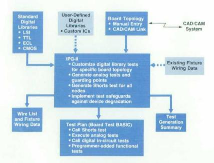
Fig. 2. The software system supplied with the HP 3065 Board Test System. IPG-II is HP's second-generation in-circuit test program generator. Requiring only board topology as its input, IPG-II uses digital test libraries and the circuit's description to generate the analog and digital in-circuit test program.
