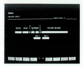
Fig. 3. Display screen for entering resistor test information.
