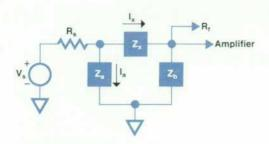
Fig. 3. One source of measurement error is introduced by source impedance  $R_{\rm s}$ .
