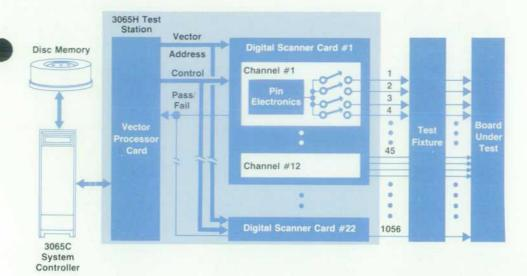
Fig. 1. Architecture of the HP 3065 Board Test System.
