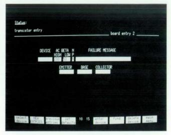
Fig. 4. Display screen for entering transistor test information.
