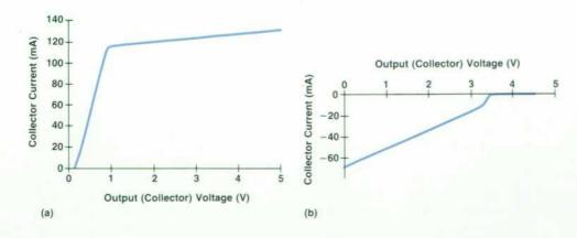
Fig. 2. Overdrive characteristics of a typical TTL LS digital device, a 74LS04 (see Fig. 3). (a) Forward characteristic for forcing an output high when the output is zero. (b) Reverse characteristic for forcing an output low when the output is a one.
