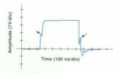
Fig. 3. Digital test stimulus waveform with glitches (indicated by arrows). If not eliminated or reduced, these glitches can cause erroneous test results.
