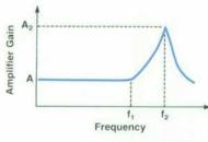
**Fig. 12.** System noise can be modeled in the measurement circuit by introducing a noise source  $E_n$  as shown in (a). Its effect on the test response is shown in (b), adding a peak at frequency  $f_2$ .
