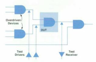
Fig. 1. In-circuit test connections to a NAND gate.
