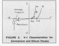
forward and reverse conductance. That is, it should show a high resistance when the diode is reversed biased and a low resistance when it is forward biased. You might wonder why the readings change
