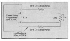
Remote sensing can correct the load-lead problem.
