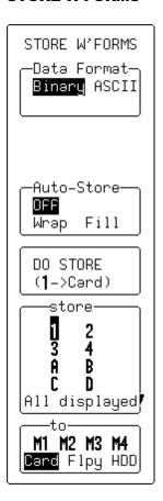
Press WAVEFORM to store waveforms to internal memory (M1, M2, M3, or M4) in LeCroy's binary format. And to store waveforms in either binary or ASCII format to floppy disk, or memory card or removable hard disk (HDD) with those options installed.
