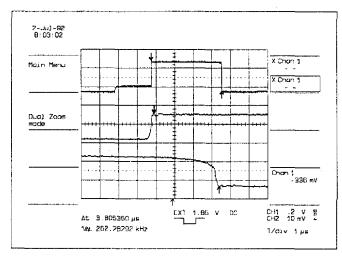
The display of acquired waveform and expanded views allows precise placement of measurement cursors and full use of the oscilloscope's 0.002% timebase accuracy.
