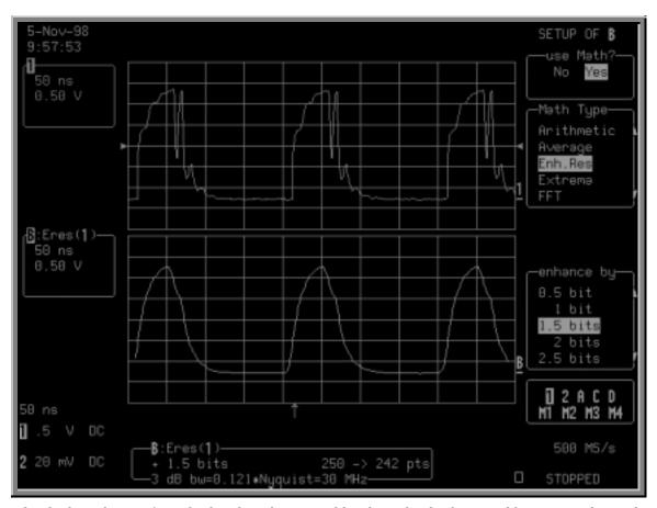
The glitch in the waveform displayed on the top grid has been clearly eliminated by ERES: the result is the waveform on the lower grid. Trace B's label indicates this as the filtered waveform. And the information field below the grids tells you that Trace B is an ERES function of Channel 1, that the waveform has been enhanced by 1.5 bits, and that filtering has reduced the number of points from 250 to 242 (see NOTE on page 131) and the bandwidth to 30 MHz.
