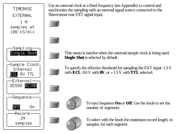
NOTE: External clock modes are available only if the EXT trigger is NOT the trigger source. Trigger time stamps and the AUTO sequence time-out feature are unavailable when you use an external clock signal. And inter-segment dead time is NOT guaranteed.
