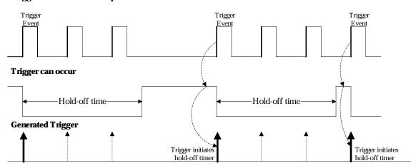
Figure 1. Edge Trigger with Holdoff by Time. The bold edges on the trigger source indicate that a positive slope has been selected. The broken upward-pointing arrows indicate potential triggers, which would occur if other conditions are met. The bold arrows indicate where the triggers actually occur when the holdoff time has been exceeded.
