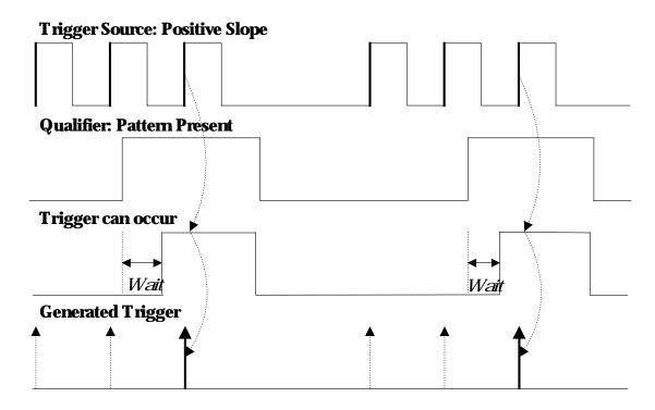
Figure 7. State Qualified and Wait: Trigger after timeout. The broken upward pointing arrows indicate potential triggers, while the bold arrows show where the actual triggers occurs.
