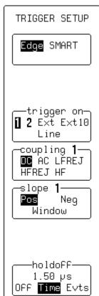
Use them to select the trigger source, the source's coupling, the slope — positive or negative — and the amount of trigger holdoff by time or events.
