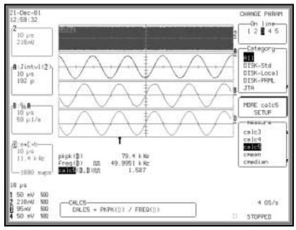
Figure 1.10. Setting Calc5 to Measure FM Modulation Index
