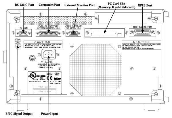
Use the RS-232-C and GPIB ports to connect your Waverunner scope to a computer or terminal, the external monitor port to display your waveforms on another monitor, and the Centronics® port to connect compatible printers or other devices. Use the PC Card slot for the PC Memory Card and portable Hard Disk options, and the BNC output for external clock signals.
