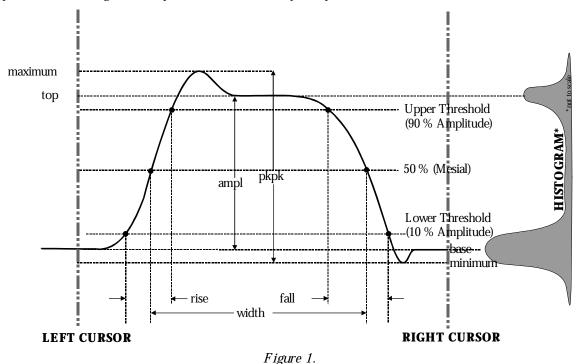
Threshold levels for rise or fall time can also be selected using absolute or relative settings (r@ level, f@ level). If absolute settings are chosen, the rise or fall time is measured as the time interval separating the two crossing points on a rising or falling edge. But when relative settings are chosen, the vertical interval spanned between the base and top lines is subdivided into a percentile scale (base = 0%, top = 100%) to determine the vertical position of the crossing points.
