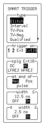
Use these menus to set up to trigger on a glitch, or to create an exclusion trigger (see page 93).
