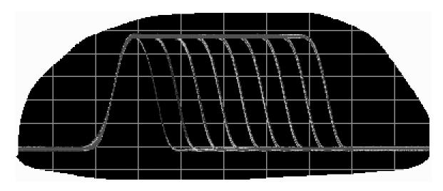
The same waveform as that shown on page 113 displayed using Color-Graded persistence shows the persistence waveform in a spectrum of colors rather than shades of a single color.
