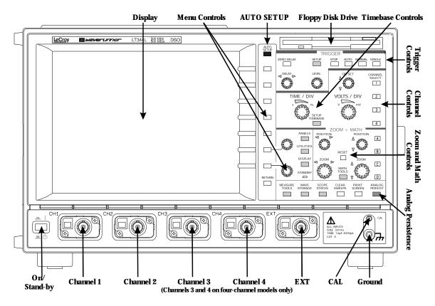
Waverunner main front panel controls and features.
