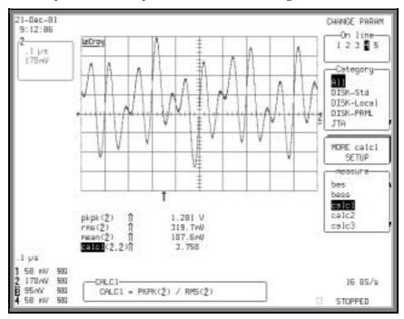
Figure 1.7. Calculated parameters allow the creation of automparameters. Here calc1 is set up to measure crest factor (peak-to-peak/rms).
