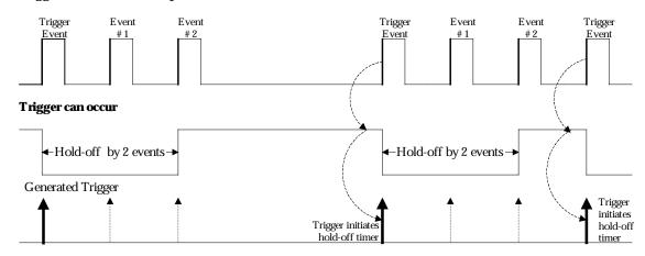
Figure 2. Edge Trigger with Holdoff by Events (in this example, two events). The bold edges on the trigger source indicate that a positive slope has been selected. The broken, upward-pointing arrows indicate potential triggers, while the bold ones show where triggers actually occur after the holdoff expires.
