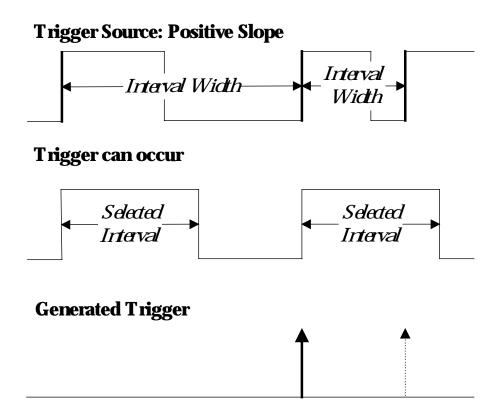
Figure 5. Interval Trigger that triggers when the interval width is larger than the selected interval. The broken upward-pointing arrow indicates a potential trigger, while the bold one shows where the actual trigger occurs — on the positive edge after the selected interval.
