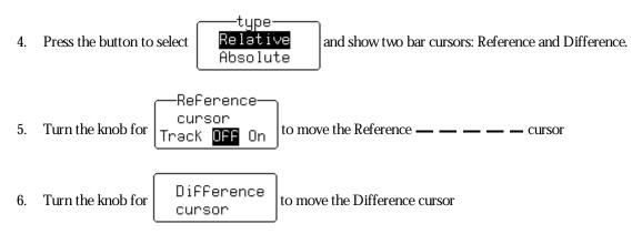
When you use Relative Amplitude cursors, the Reference cursor can be made different from the ground level. You might place it, for example, at the base level of a square wave. You could then position the Difference cursor at the top of the waveform. The difference between the two would then give you the signal's amplitude, indicated in the trace label, as illustrated on the next page.
