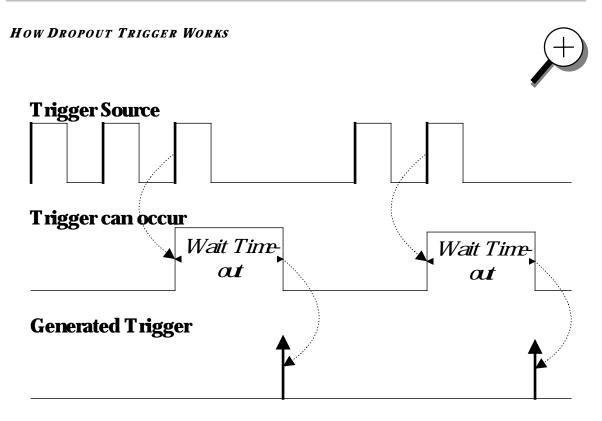
Figure 9. Dropout Trigger: occurs when the timeout has expired. The bold upward-pointing arrows show where the trigger occurs.
