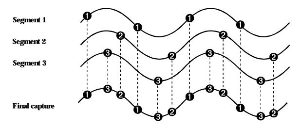
Figure 1. Buildup of an RIS waveform.
