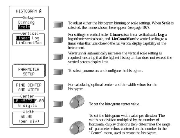
Figure 2.1, below, shows the display when "Histogram" is selected from the "Math Type" menu. The freq parameter only has been defined. To define additional parameters, select from the "Histogram custom line" menu.
