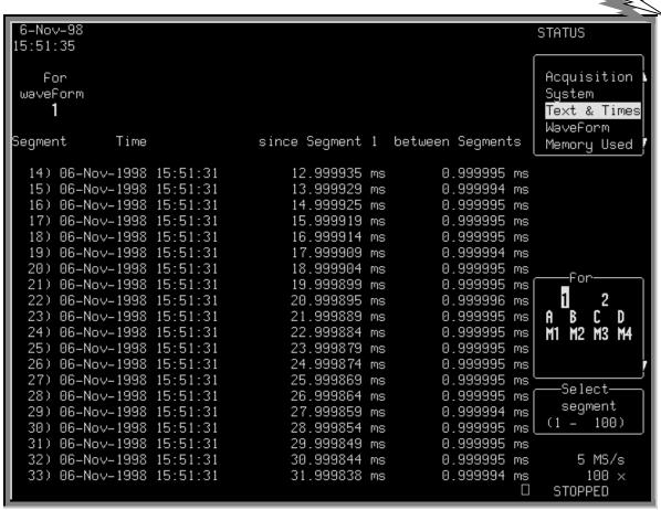
Press the SCOPE STATUS button for a full status summary of your sequence acquisition. Use the Select segment menu and its button and knob to scroll down the segment list.
