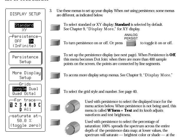
TIP: At 0% intensity in Standard display without persistence, the waveform and text disappear:
