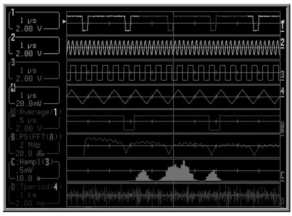
Waveform source descriptions, trace labels and the information they contain will always take the color of their respective traces, as in this four-channel model's Octal-grid, eight-trace display.
