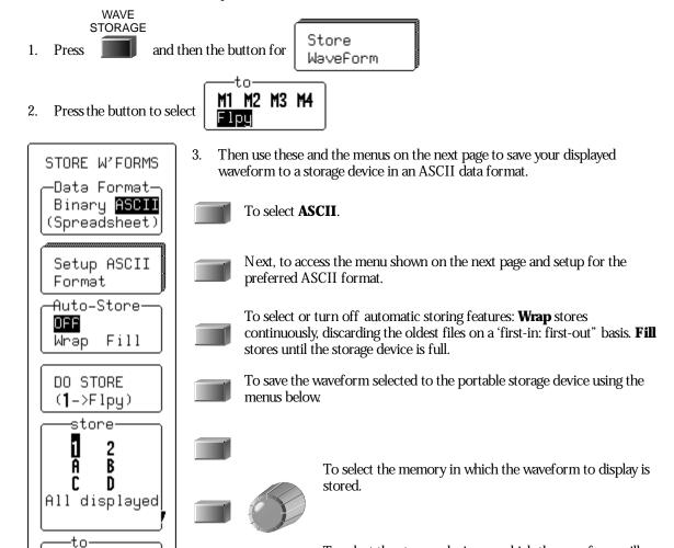
To select the storage device on which the waveform will be stored: floppy disk (**Flpy**) is standard on all Waverunner models, while a PC memory card or hard disk card in the rear PC Card slot (**Card**) is an option.
