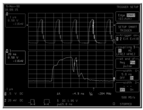
Trigger on a glitch of width  $\leq 5.0$  ns on the negative slope. Here, the glitch is marked by arrow cursors on the waveform. Trace A on the lower grid is a zoom of the waveform on the top grid. Information on the trigger is given beneath the grid.
