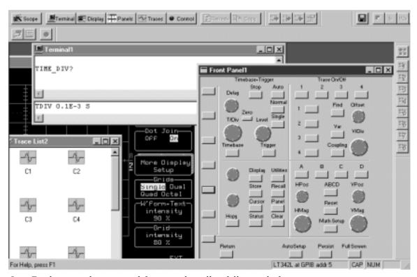
ScopeExplorer now has a virtual front panel to allow full control of remote scopes.
