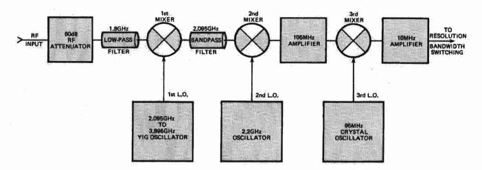
Fig. 1. Frequency conversion system of the 7L13.
