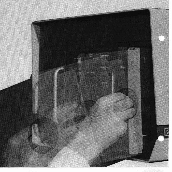
in 100-ns increments, are available in this mode. A helidial-controlled analog delay provides an additional 0 to 100 ns of delay providing time delay resolution up to 1 ns.
