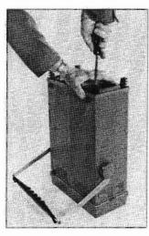
Fig. 1. The 465 cabinet is removed by loosening six screws on the rear panel. earlier instruments, take care that the cabinet clears the components on the trigger-view board. In later instruments this circuitry is laid out on the trigger board.
