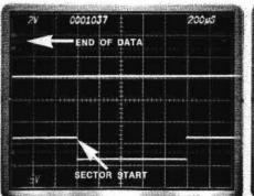
Fig. 5. Time interval from end of data in one sector to start of next sector pulse is easily viewed with the 7D11.
