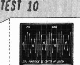
The readout in this photo was programmed by the computer in a Digital Processing Oscilloscope system. The double V indicates the waveform is the resultant of two voltage signals multiplied together. This photo was dated and identified as
