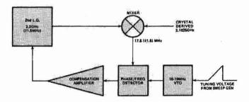
Fig. 2. Second L.O. stabilization system.
