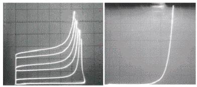
(a) 2N2222 NPN BJT (b) 1N4152 diode Fig. 1: Curves Of (a) npn Bipolar Junction Transistor (BJT), (b) Diode
