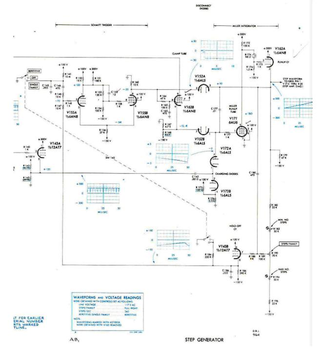
Fig. 3: The Tek 575 Step Generator Circuit Diagram © 1960 Tektronix, Inc., Reproduced with Permission. All Rights Reserved
