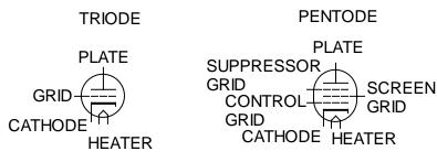
Fig. 4: Schematics Used For Triode And Pentode With Connections
