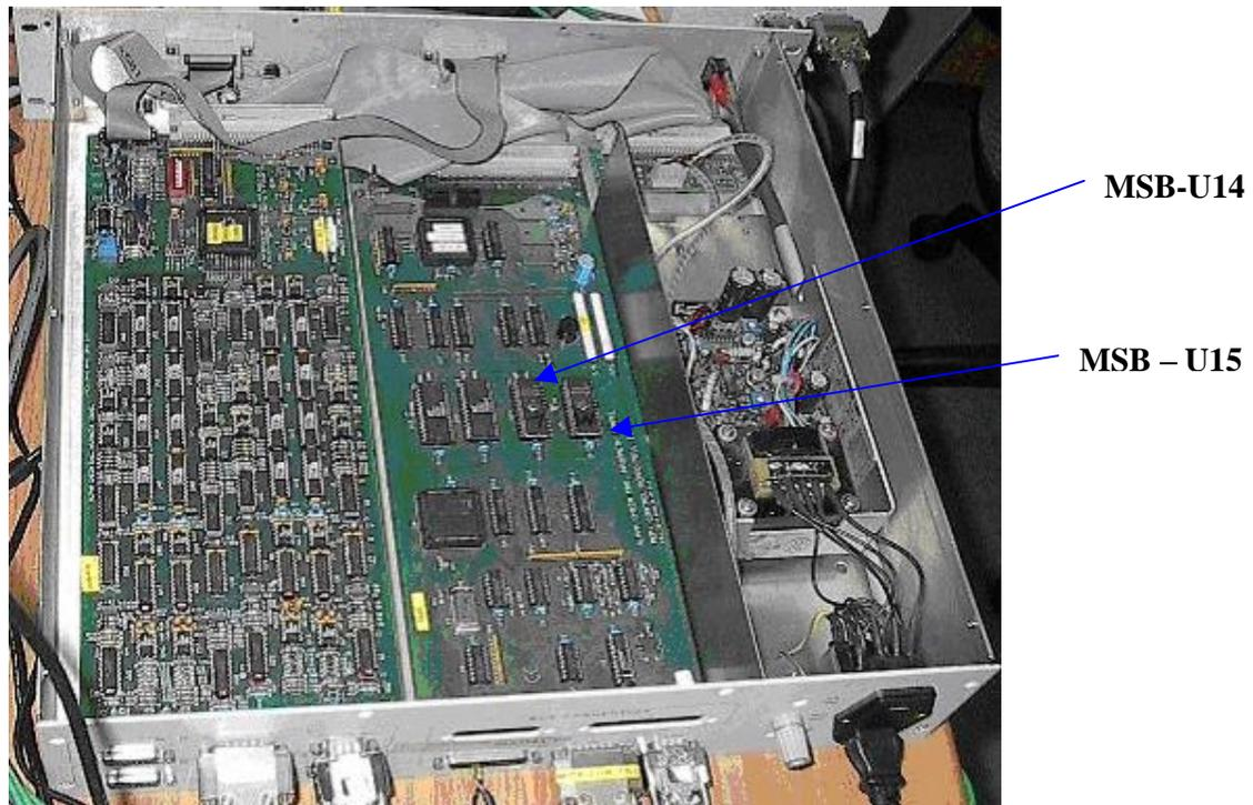
4. Install new PLM chips. Please note, every bank has label MSB or LSB. The same labels there are on every chip. Every chip should be inserted accordingly. Polarity of chips is important – please note small notch on chip and its bracket.
