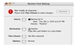
Check over the various parts of this window. Make sure the destination volume is correct and you are copying files and folders to a new folder. Note that no files are currently selected, which is why the summary says the operation is "Not ready to execute."
