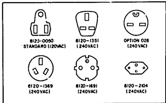
Figure 2-2. Power Cord Plug Configurations
