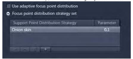
13 To change the Focus point distribution strategy set, double-click on the entry. A window comes up, in this window you can select another Focus point distribution strategy set via the dropdown menu and you can adjust the parameters for this setting. With a click on Modify the changes will be applied.
