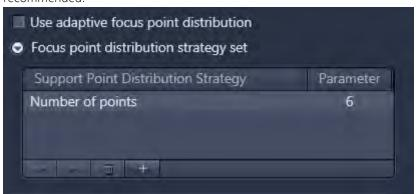
**14** To change the **Focus point distribution strategy set**, double-click on the entry. A window comes up, in this window you can select another Focus point distribution strategy set via the dropdown menu and you can adjust the parameters for this setting. With a click on **Modify** the changes will be applied.
