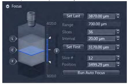
Once the specimen is in focus, double-check that the image is not too bright or too dark. If you need to adjust one of these parameters, please change the settings under Exposure. By clicking on the Measure button, the system will automatically determine the best Flash intensity and Flash duration. For best results, move the stage to a position that keeps specimens out of the light path.
