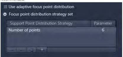
9 To change the Focus point distribution strategy set, double-click on the entry. A window comes up, in this window you can select another Focus point distribution strategy set via the dropdown menu and you can adjust the parameters for this setting. With a click on Modify the changes will be applied.
