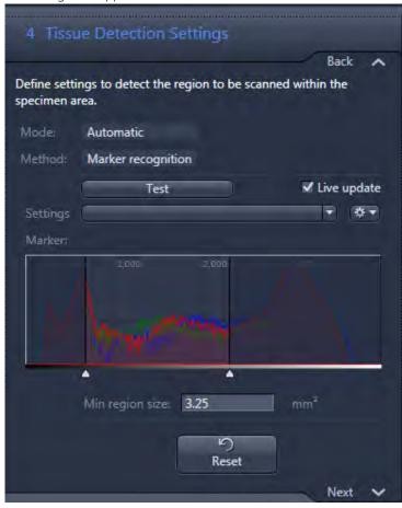
The settings are limited to the definition of the marker threshold (comparable to the tissue threshold described above). The only further adjustable value is the **Min region size**, whose functionality is the same as described above.
