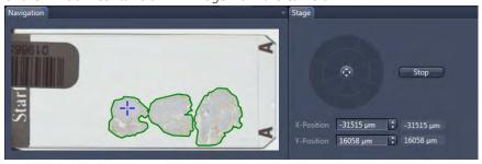
3 To be able to judge the quality, you first have to focus (using the Focus expander). This section is only for focusing and has no influence on the focusing in the subsequent scan as the settings have already been made in the previous step. Use the Run Auto Focus button to focus automatically. If the autofocus is running you can interrupt the focus run by clicking on Stop Auto Focus.
