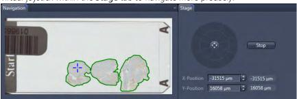
4 The next step is to adjust the *Sharpness measure set* [▶ 61]. For the 2.5x objective **FFT** is the best choice for the coarse focus in RAC for the other objectives (5x and 10x) use Basic or Best only in case if this does not work use **FFT**.
