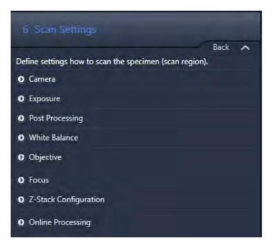
Here you can set up the scan settings. These settings are important as they determine the image quality that is subsequently experienced by the user in terms of exposure time, white balance, etc. The settings under **Post Processing** and **White Balance** are similar to the standard ZEN tools.
