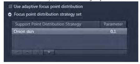
9 To change the Focus point distribution strategy set, double-click on the entry. A window comes up, in this window you can select another Focus point distribution strategy set via the dropdown menu and you can adjust the parameters for this setting. With a click on Modify the changes will be applied.
