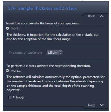
Based on this thickness, the software will calculate the number of focus levels and the distance of these levels based on the objective used. Finally, you can decide if the z-stack should be conserved or if an **EDF**
