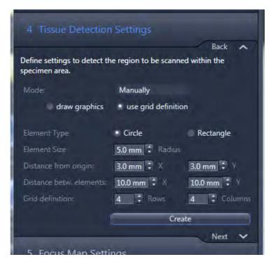
You can define a grid with rectangles or circles as **Element Types** in a regular pattern. The reference point for this grid is the upper right-hand corner of the specimen area (red rectangle). Based on this, you can define on offset from the upper left-hand corner in x (A) and y (B) in mm and also the pitch of the grid in x (C) and y (D).
