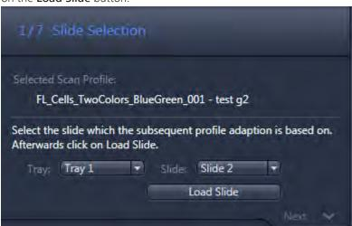
**3** The first step is the **Slide Selection**. Select the **Tray** and **Slide** position and click on the **Load Slide** button.
