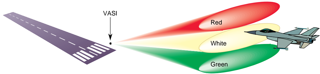
Figure 17-1 VASI Landing Light
