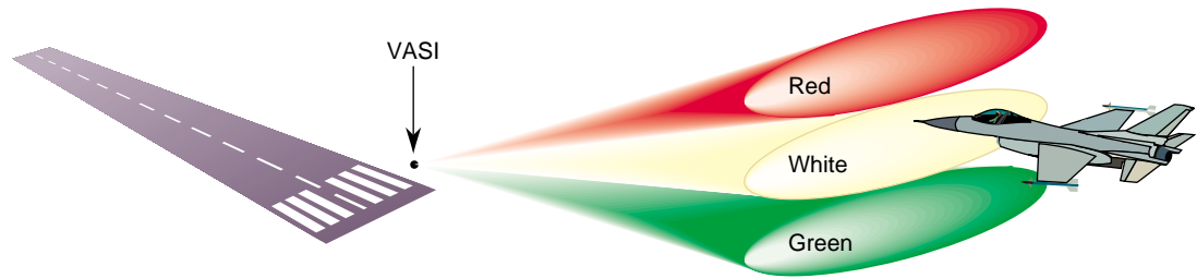
Figure 18-1 VASI Landing Light
