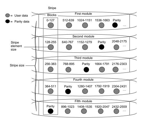
Figure 1-13 Distribution of User and Parity Data in a RAID-5 Group
