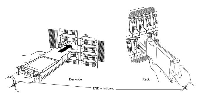
Figure 5-9 Inserting the Replacement Disk Module
