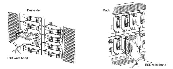
Figure 5-5Pulling Out a Disk Module
