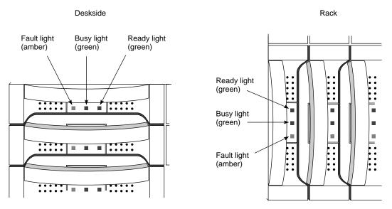
Figure 1-9 Disk Modules and Status Lights
