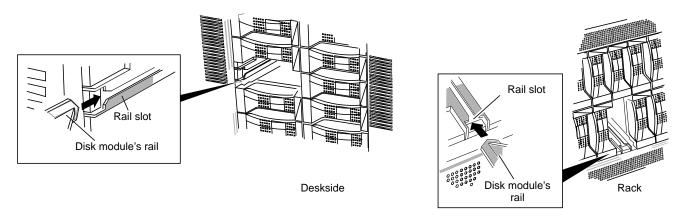
Figure 5-7 Engaging the Disk Module Rail
