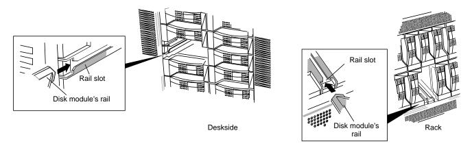
Figure 5-12 Engaging the Disk Module Rail
