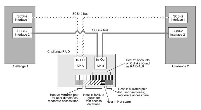
Figure 2-3 Dual-Bus/Dual-Initiator Configuration Example
