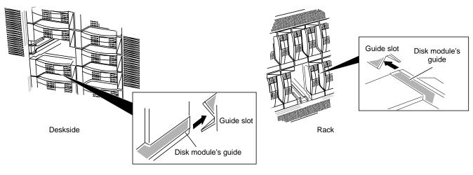
4. Engage the disk module's guide in the chassis guide slot, as shown in Figure 5-8.
