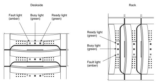
Figure 5-1 Disk Module Status Lights
