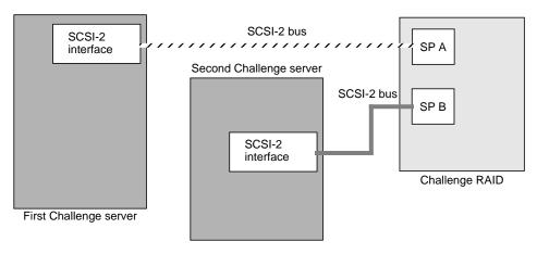
Figure 1-6 SPs Connected to Different Challenge Chassis
