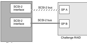
Note that the disk modules are owned by the SP, and not by the host, the SCSI-2 bus, or the storage system.
