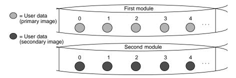
Figure 1-10 RAID-1 Mirrored Pair (Hardware Mirrored Pair)
