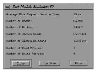
Figure 3-9 Example Disk Module Statistics Window
