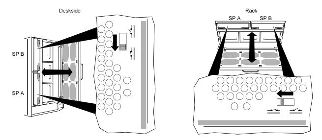
4. For the AMD-based SP, move the SP's power switch to the enable position, as shown in Figure 3-23.
