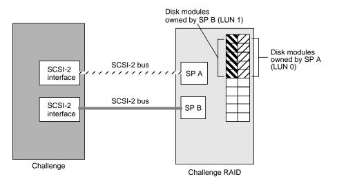
Figure 2-1 Dual-Interface/Dual-Processor Configuration Example
