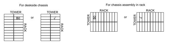
Figure 5-11 Marking the Label for Disk Module B0
