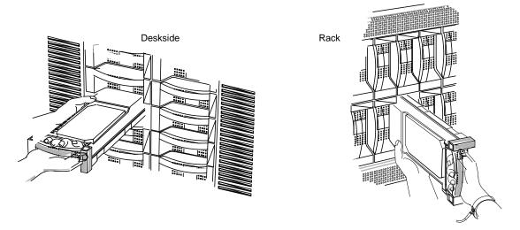
Figure 5-6 Removing a Disk Module
