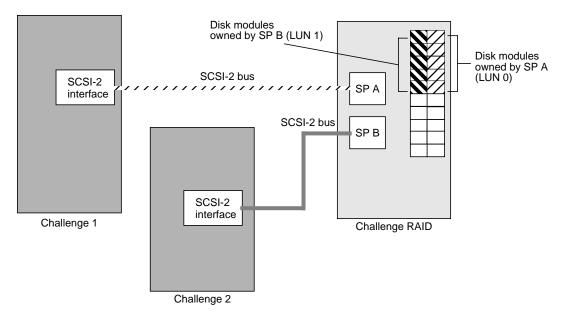
**Figure 2-2** Split-Bus Configuration Example
