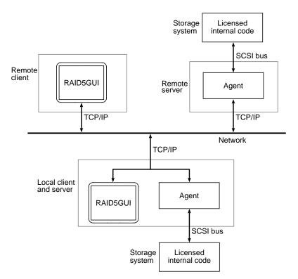
Figure 1-15 RAID5GUI Management Environment Architecture
