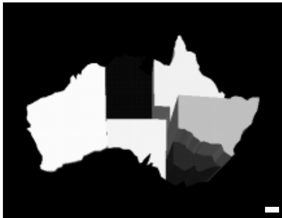
Figure 1-26 Representation of a Null Value Mapped to Height (Top Middle Object) and to Color (Bottom Right Object)
