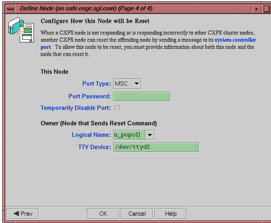
Figure 10-7 Example System Controller Settings
