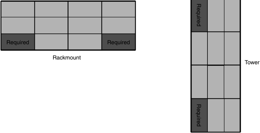
Figure 1-19 Required Disk Drive Module Locations
