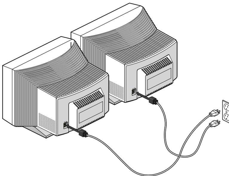
**Figure 2-3** Connecting the Power Cables
