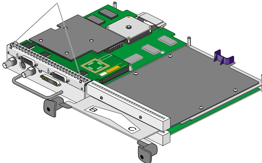
**Figure 1-18** VPro Locator Tabs Protrude through Display Option Board Locator Slots
