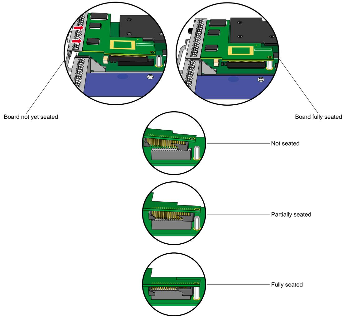
**Figure 1-17** Seating the Display Option Board On the VPro Graphics Board (side view)
