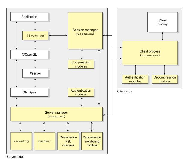
Figure 3-1 Overall Diagram of OpenGL Vizserver
