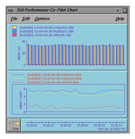
Figure 3-3 pmchart Using OpenGL Vizserver PMDA
