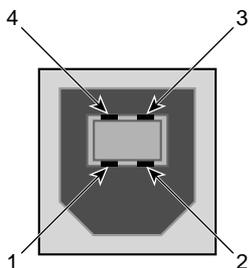
**Figure A-11** Pin Number Locations for USB Type B Connector
