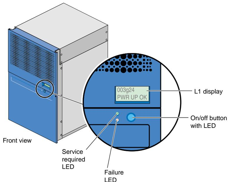
**Figure 5-2** Front Components
