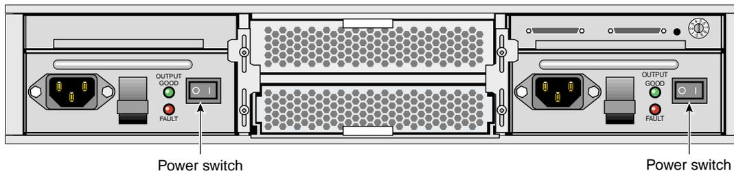
**Figure 2-5** TP900 Power Switch (| Position)
