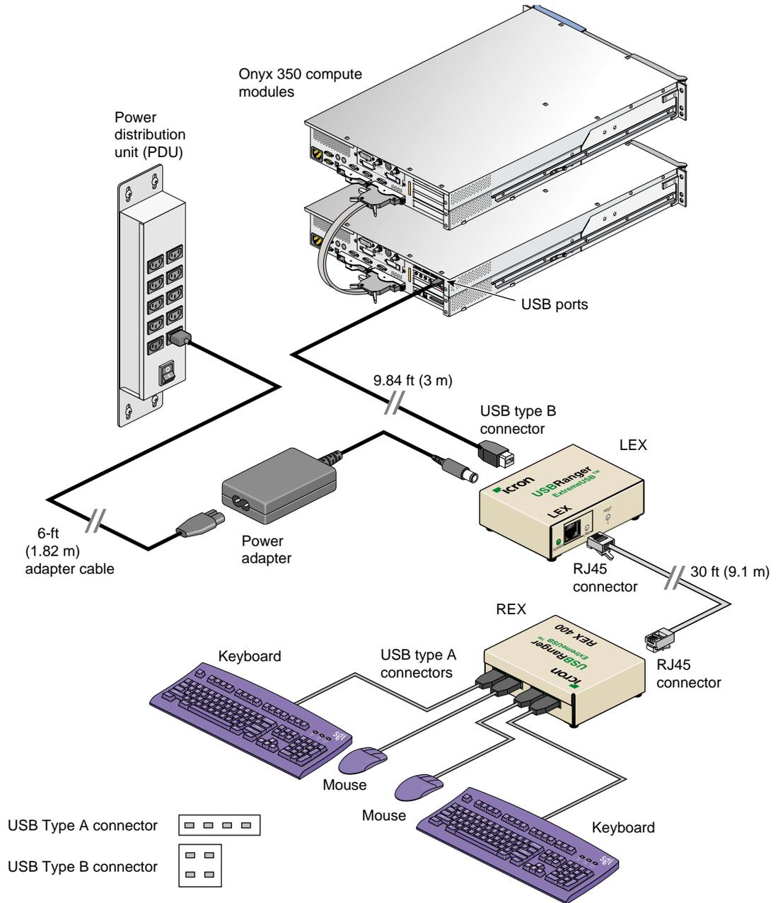
**Figure 2-4** Keyboard and Mouse Connected via Optional USB Extender
