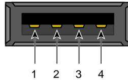
**Figure A-5** USB Hub Type A Connectors
