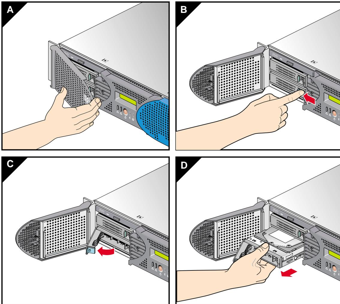
**Figure 7-14** Removing a Disk Drive
