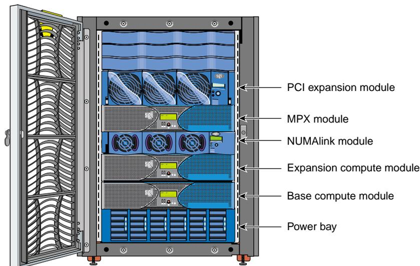
**Figure 3-9** System with Base Compute Module, System Expansion Compute Module, MPX module, and 4U PCI Expansion Module
