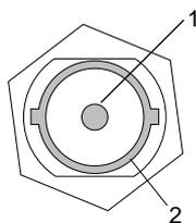
**Figure 4-3** Genlock Port Pinouts
