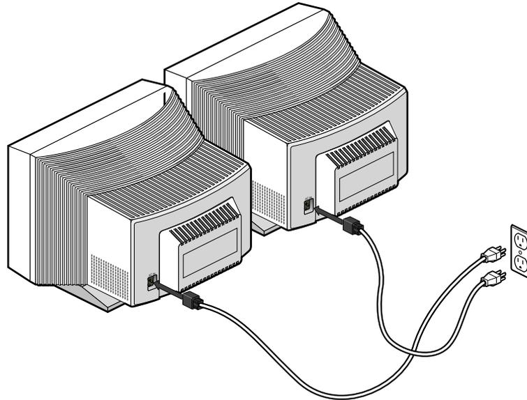
**Figure 4-9** Connecting the Monitor Power Cables
