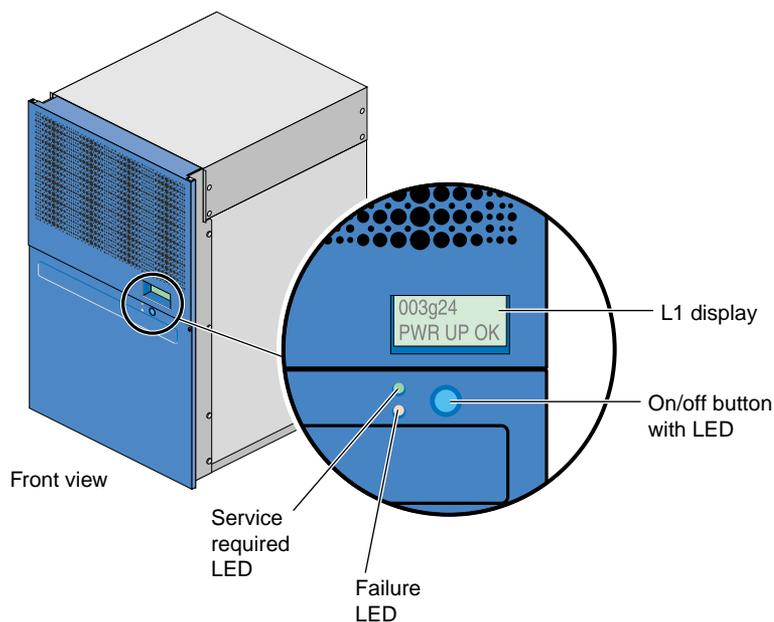
**Figure 5-9** L1 Controller Display, On/Off Button, and LEDs
