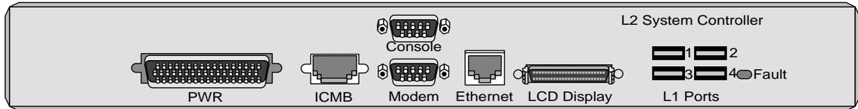
**Figure A-2** Non-proprietary Connectors on Rear Panel of L2 Controller
