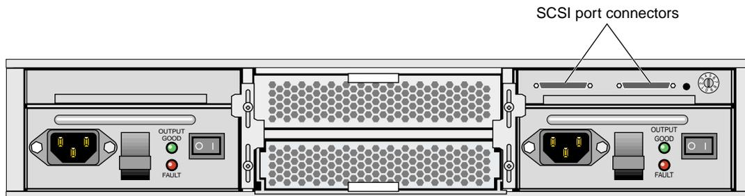
**Figure A-4** Non-proprietary Connectors on Rear Panel of TP900 Storage Module
