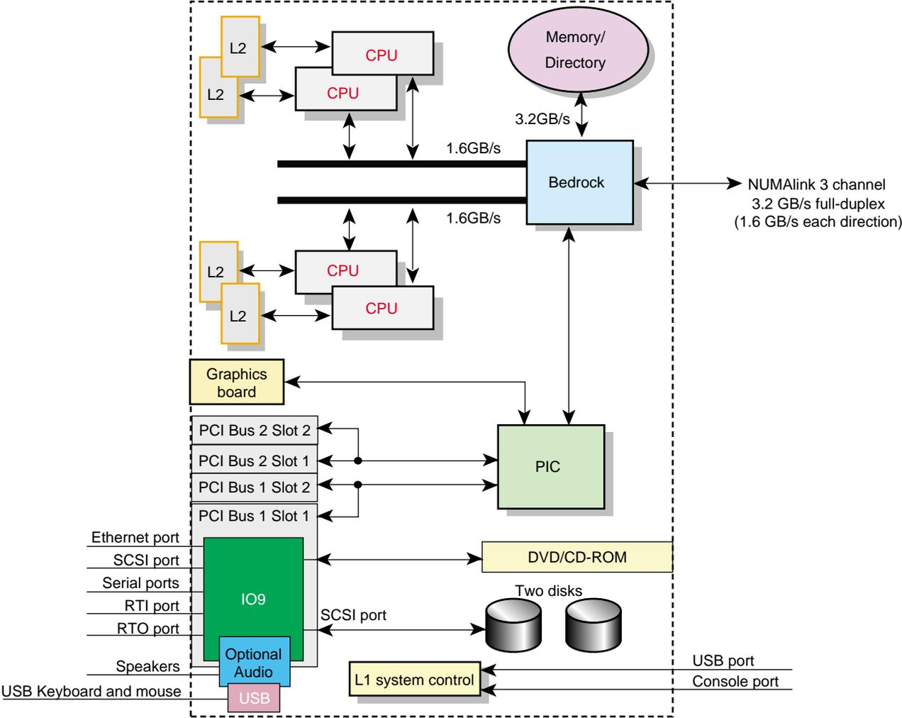
Figure 1-2 Functional Block Diagram of a Basic IP Graphics System
