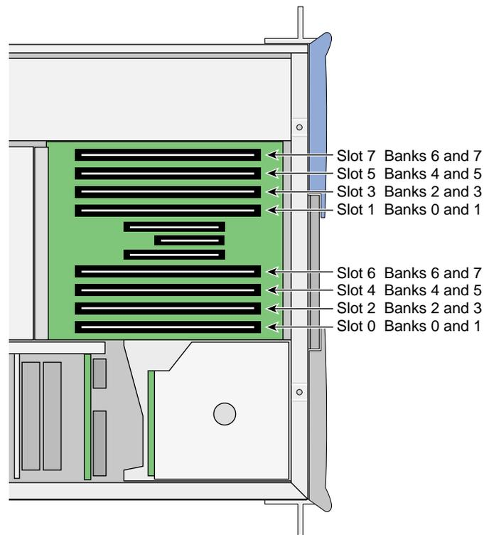
**Figure 7-15** Layout of DIMM Slots and Local Memory Banks
