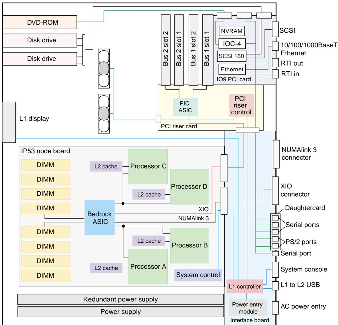
**Figure 3-2** Block Diagram of a Base Compute Module
