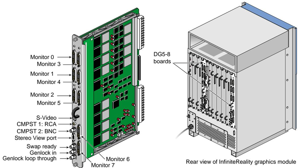
**Figure 5-8** DG5 (Display Generator) Board
