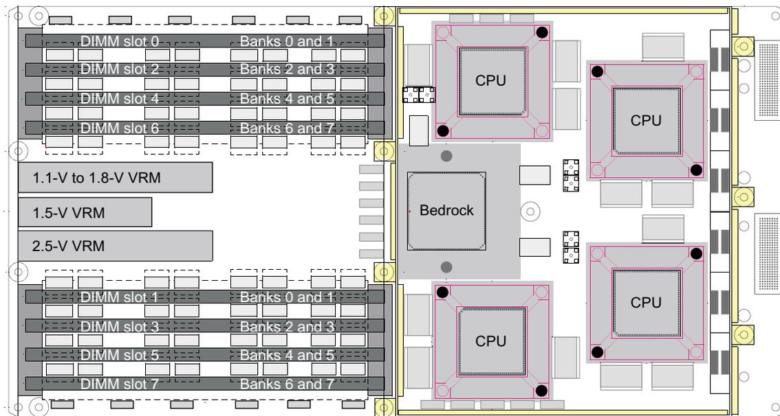
**Figure 3-7** Layout of DIMM Slots and Local Memory Banks
