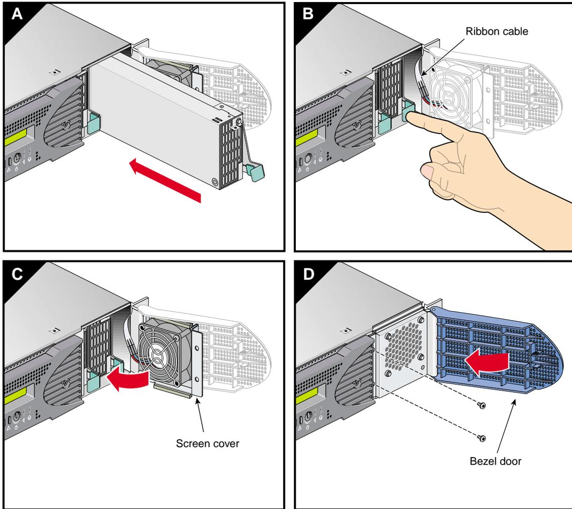
**Figure 7-28** Example of Power Supply Replacement
