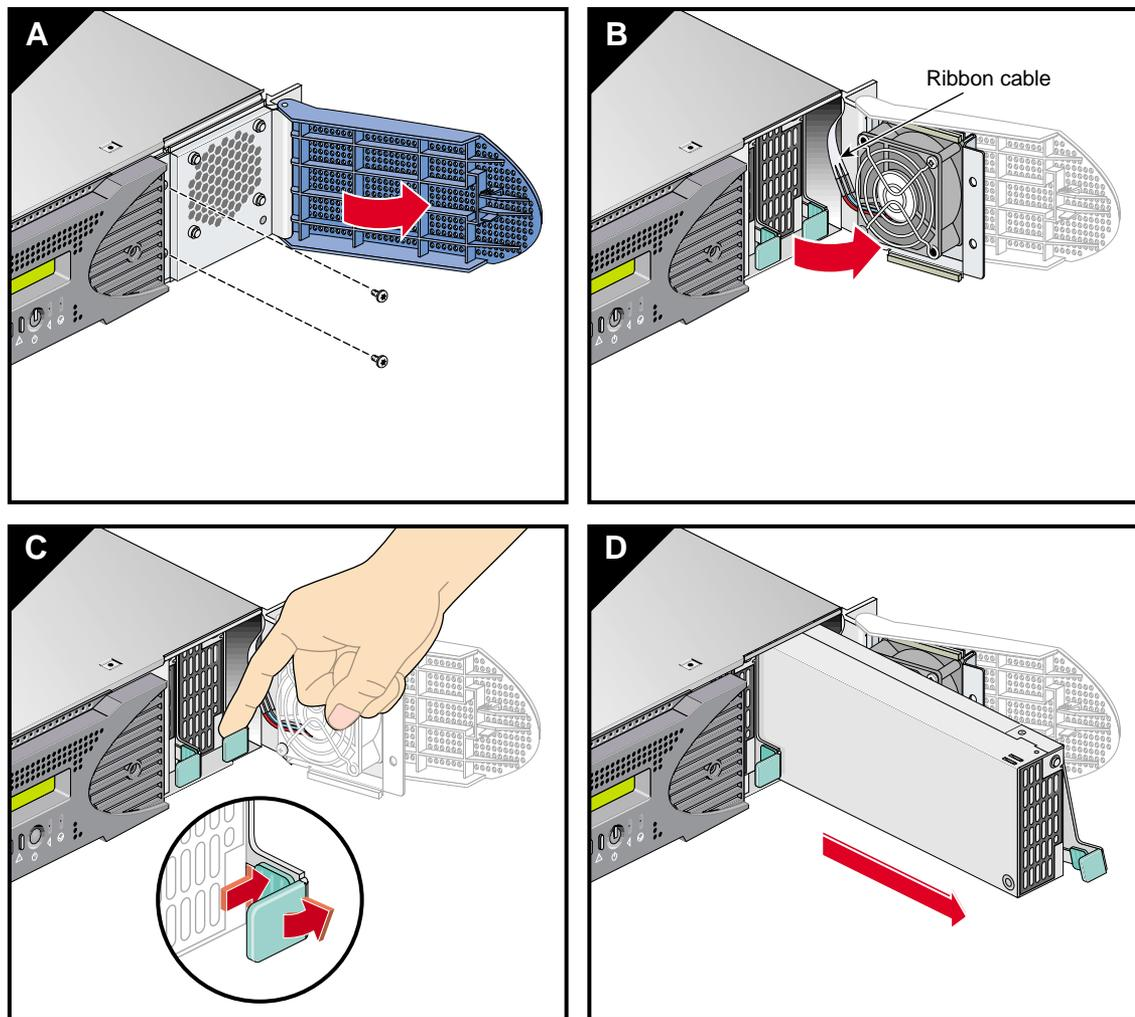
**Figure 7-27** Removing a Power Supply
