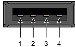
**Figure A-10** Pin Number Locations for USB Type A Connector
