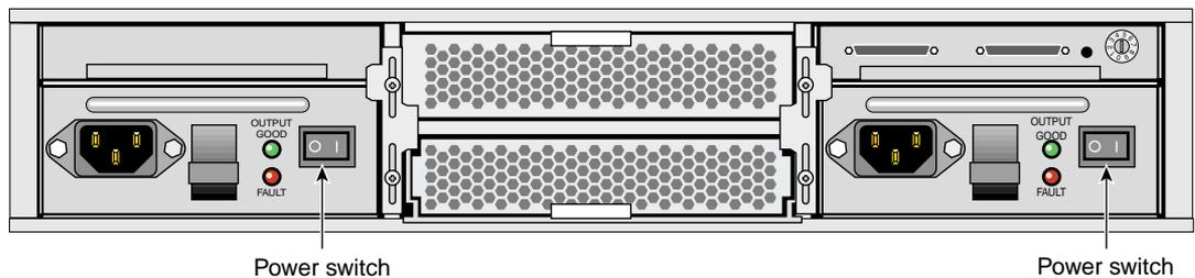
**Figure 2-13** TP900 Power Switch (**0** Position)
