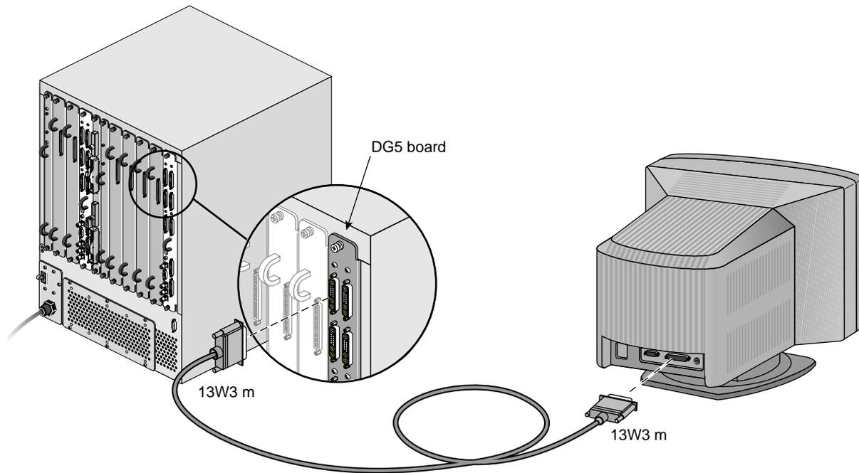
**Figure 2-1** InfiniteReality Monitor-to-DG5 Connection
