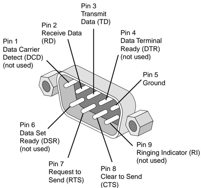
**Figure A-6** DB9 Connector Pin Assignments
