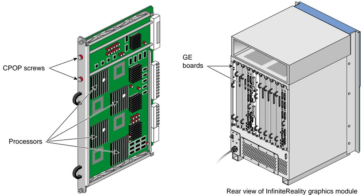
**Figure 5-6** GE (Geometry Engine) Board
