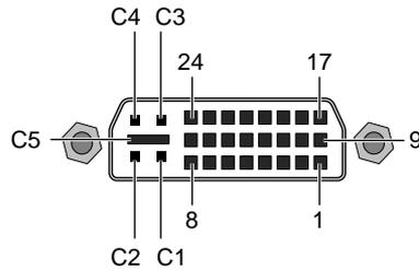
**Figure 4-6** DVI-I Port and Pinouts
