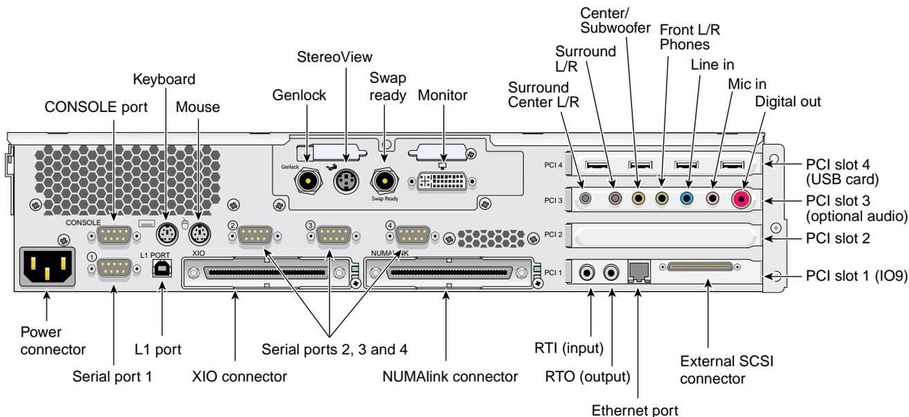
**Figure 4-1** InfinitePerformance, IO9, USB, and Optional Base Audio in the Base Module
