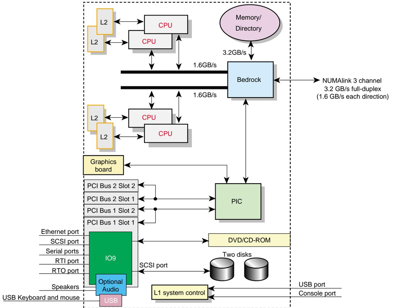
**Figure 4-2** Block Diagram of the Onyx 350 Graphics and Compute Module
