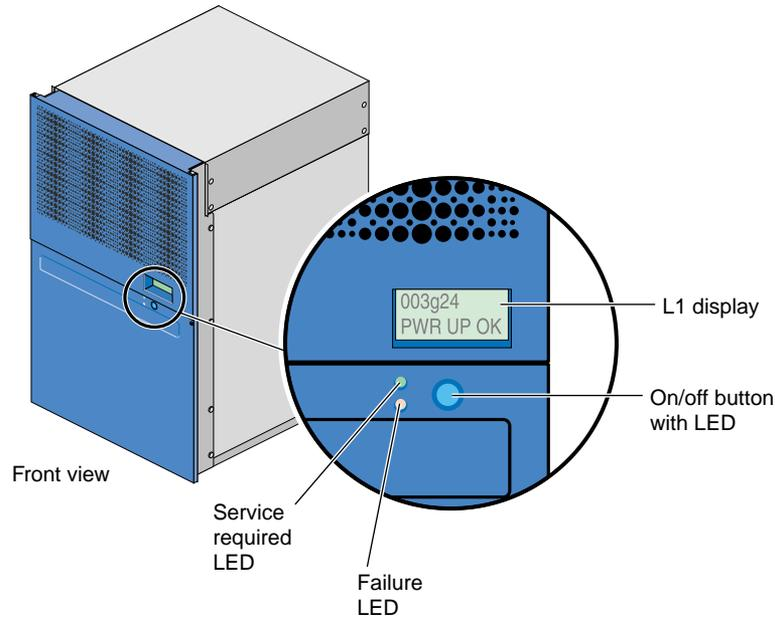
**Figure 2-12** Front View of InfiniteReality Graphics Module
