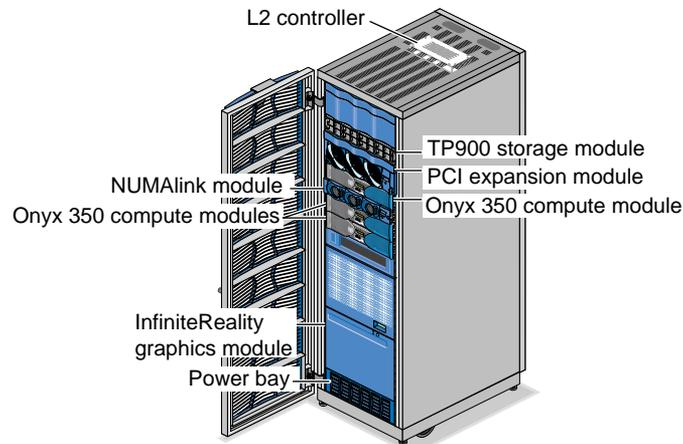
**Figure 1-1** Example of Onyx 350 InfiniteReality Visualization System
