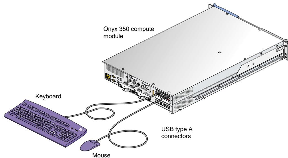
**Figure 2-3** Keyboard and Mouse Connected Directly to Compute Module
