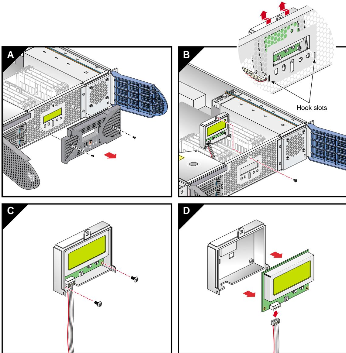
**Figure 7-24** Removing the L1 Controller Display Panel
