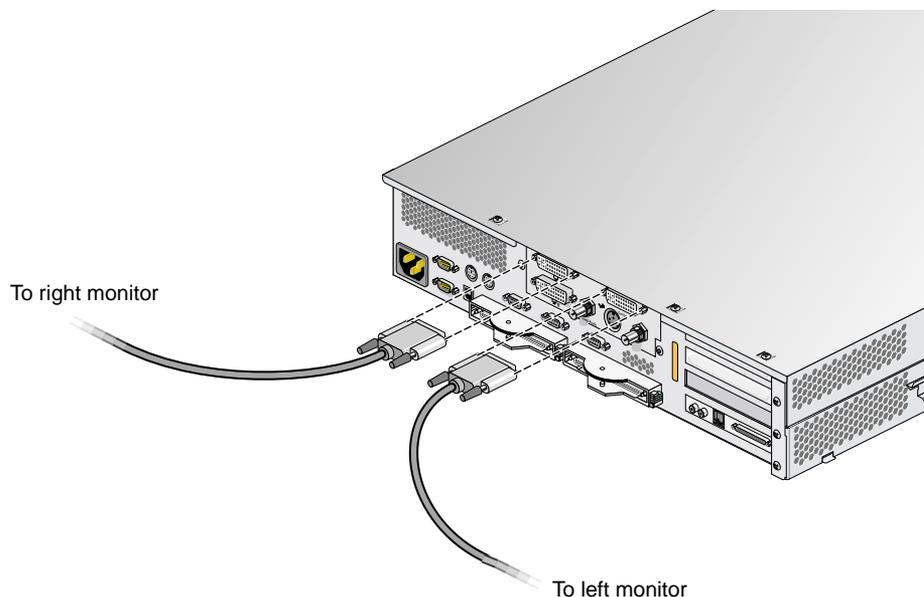
**Figure 4-8** Connecting the Monitor Signal Cables to the DCD
