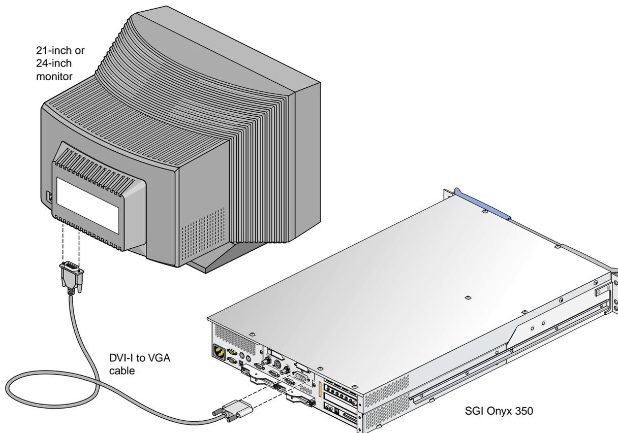
**Figure 2-2** Connecting InfinitePerformance DVI-I to a Monitor
