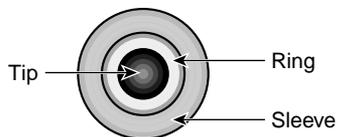
**Figure A-9** Stereo Jack Connector Conductor
