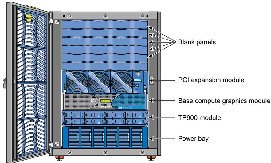
**Figure 3-8** System with One Base Compute Module, One 4U PCI Expansion Module, and One TP900 Module
