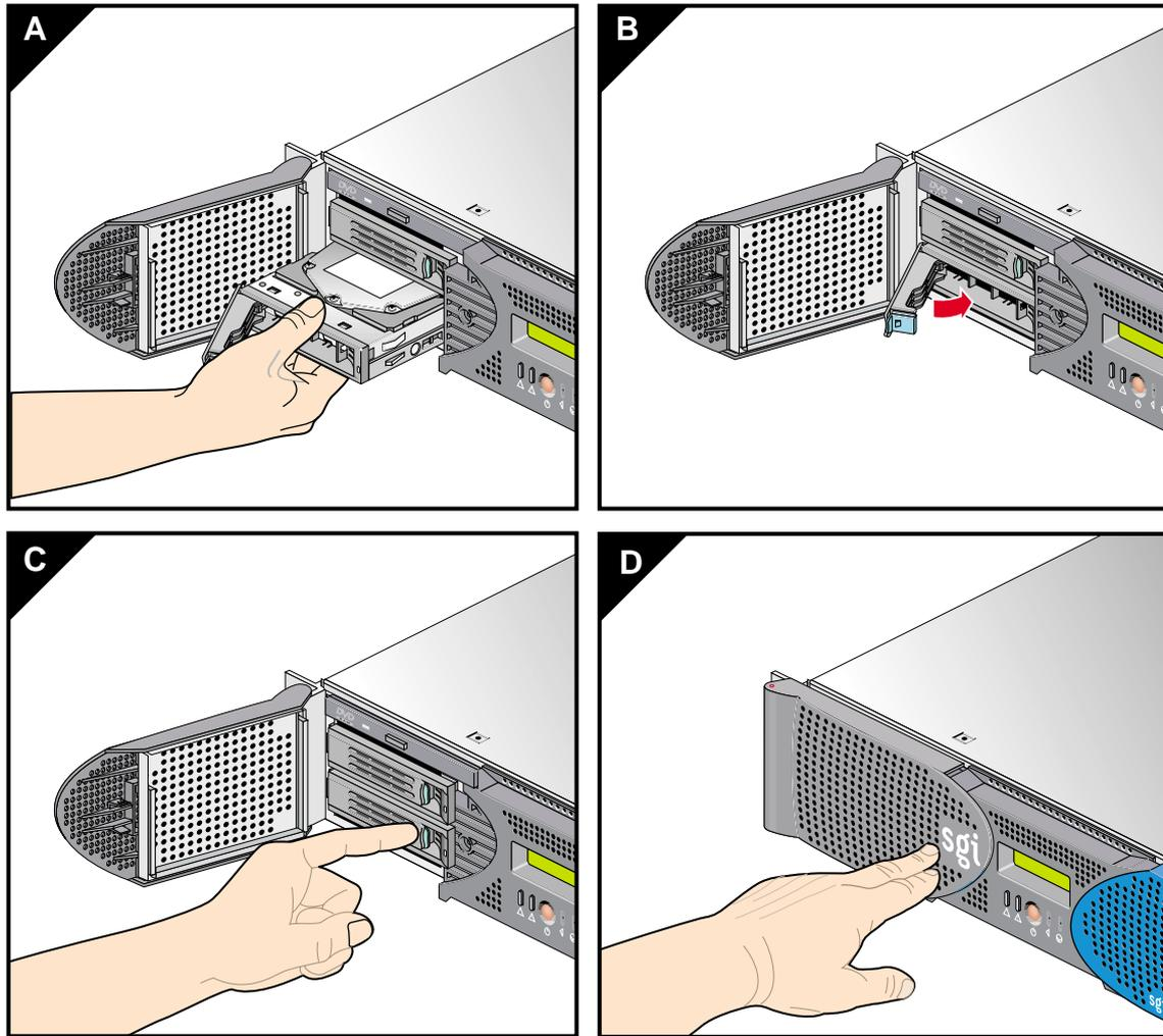
**Figure 7-13** Installing a Disk Drive
