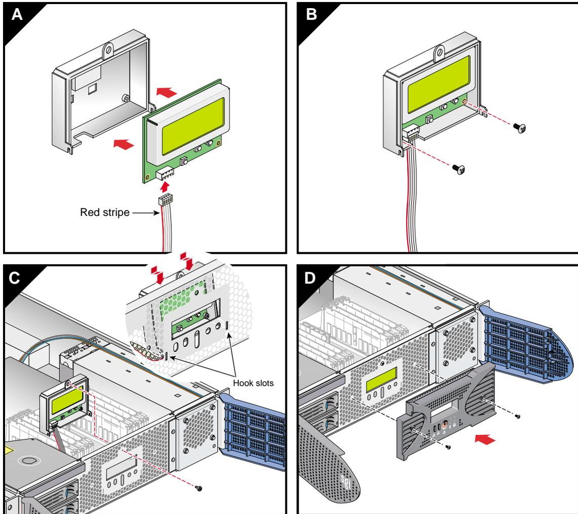
**Figure 7-25** Installing an L1 Controller Display Panel
