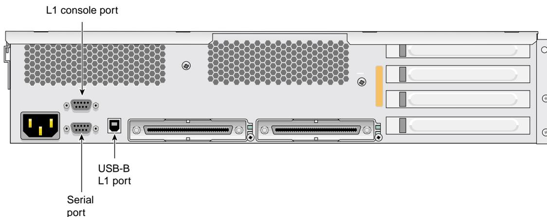
**Figure A-1** Non-proprietary Connectors on Rear Panel of MPX Module
