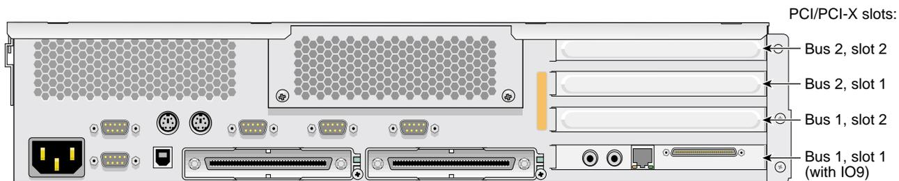
**Figure 7-3** PCI and PCI-X Card Slots Located in the Rear Panel of the Module
