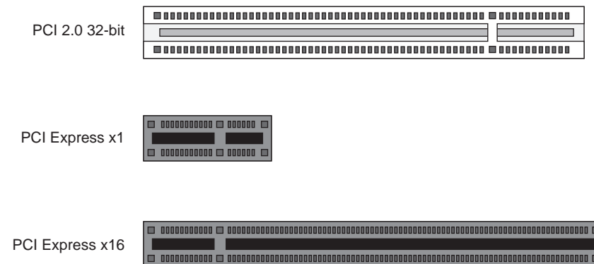
Figure 5-1 Comparison of PCI/PCI-X Connector with PCI Express Connectors
