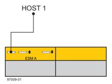
Figure 3–2 Single ESM, Single Host, and Multiple Storage Enclosures
