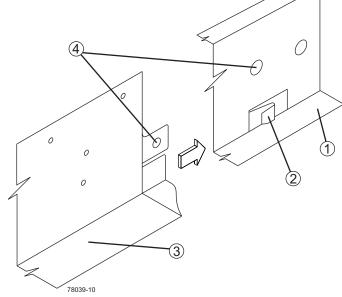
Figure 2–5  $\,$  Sliding the Storage Enclosure into the Clip on the Mounting Rail
