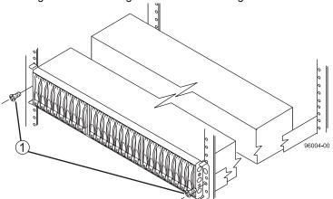
Figure 2-6 Attaching the Front of the Storage Enclosure
