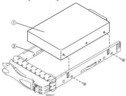
Figure 2-8 Installing a Drive in a Drive Canister
