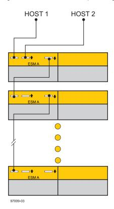
Figure 3–3 Single ESM, Dual Host, and Multiple Storage Enclosures
