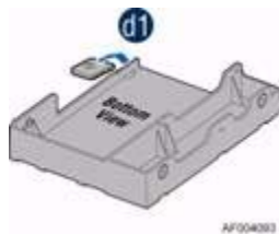
Figure 4-13 Breaking Tab on HDD Interface Bracket
