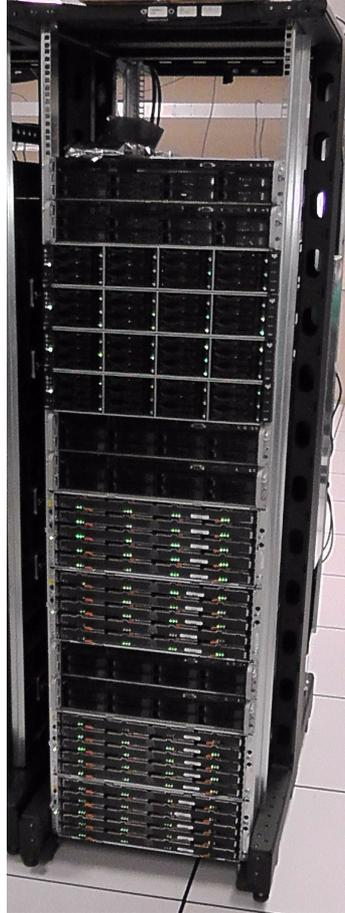
**Figure 2-6** I/O Expansion Rack
