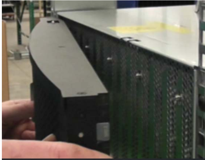
Figure 1-3 Attaching the Left Side of the Front Grille to the Chassis
