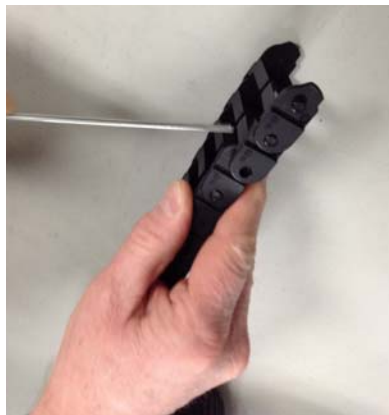
Figure 1-50 Pry the Joint Apart
