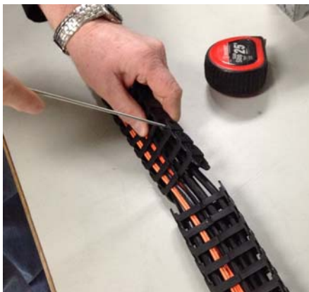
Figure 1-56 Pry Apart the Joint at the Other End
