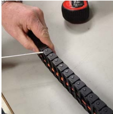
Figure 1-53 Remove Segments from the Middle of a Full Arm
