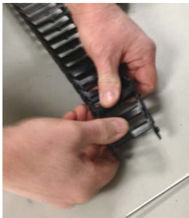
Figure 1-51 Pull the Segments from the Arm
