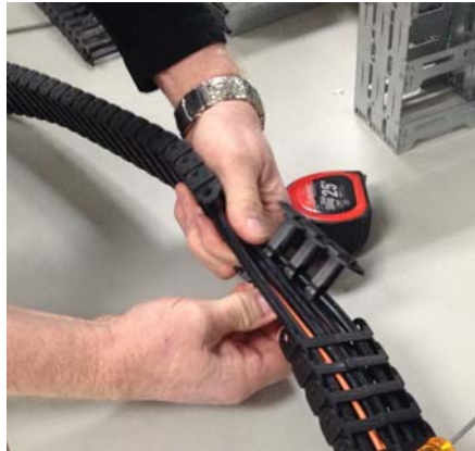
Figure 1-57 Twisting the Section of Segments from the Cables
