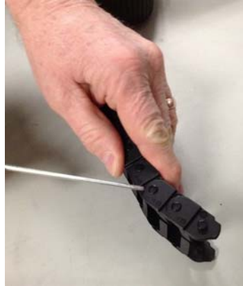
Figure 1-49 Remove Segments from the End of an Empty Arm
