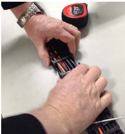
Figure 1-55 Pull Apart the Cable Management Arm
