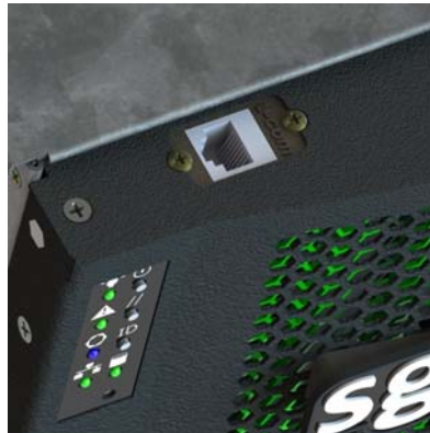
Figure 1-77 MIS-S9D Proprietary Network Interface
