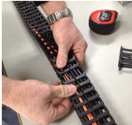
Figure 1-58 Join the Spliced Ends of the Cable Management Arm
