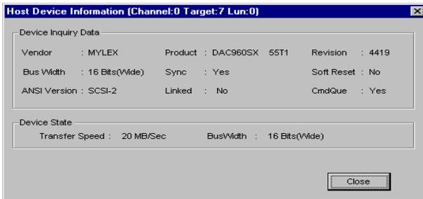
**Figure 5-13. Host Device Information: RAID Controller**
