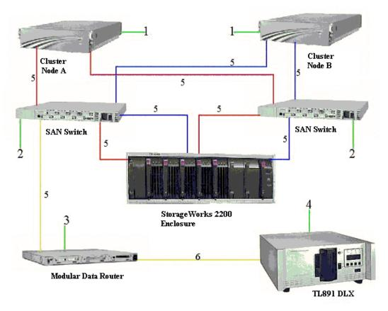
Figure 3: Cabling the Modular Data Router
