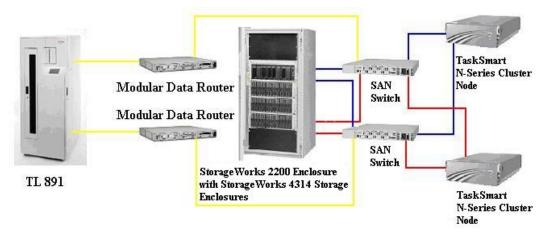
Figure 1: Compaq TaskSmart N-Series Cluster environment
