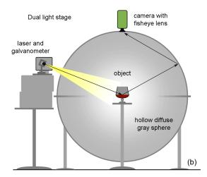
**Figure 1:** (a) A traditional light stage, where an object is progressively photographed as illuminated by a number of lighting directions. (b) A dual light stage, where a laser is scanned across the object and the scattered light forms images on the inside of a diffuse sphere. The reflectance function images are recorded by a camera with a fisheye lens that views the entire sphere.
