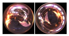
**Figure 4:** A light probe image in angular map format (left), and our fisheye lens representation (right).
