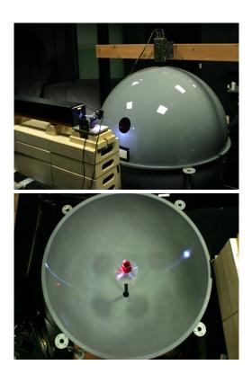
**Figure 2:** (a) A dual light stage comprises a sphere, a laser, a 2-axis galvanometer scanner, and a video camera. (b) The top half of the sphere has been removed to show the object inside. We can see the patterns of reflected light on the inside of the sphere.
