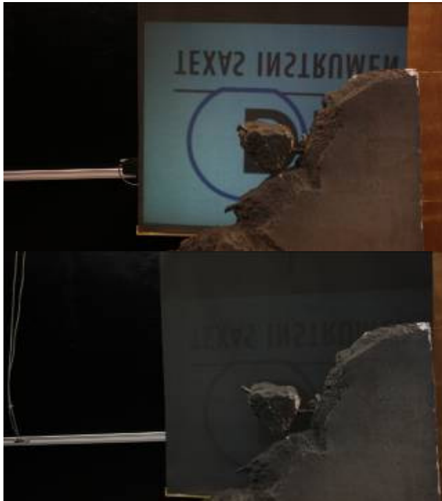
Figure 4: Retroreflected illumination level near the optical axis of the micro-projector (above) and the retroreflected illumination at 16 inches from the optical axis (below) with screen placed behind concrete wall prop.
