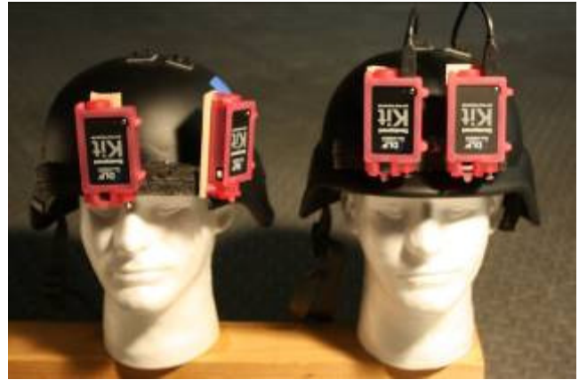
Figure 5: A projector configuration for a wider field of view (left) or for 3D stereoscopic imagery (right).
