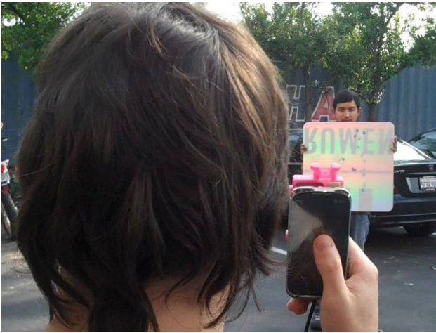
Figure 7: Near-axis view cast in daylight test of retroreflective sign material as seen by user holding projector/mobile phone.
