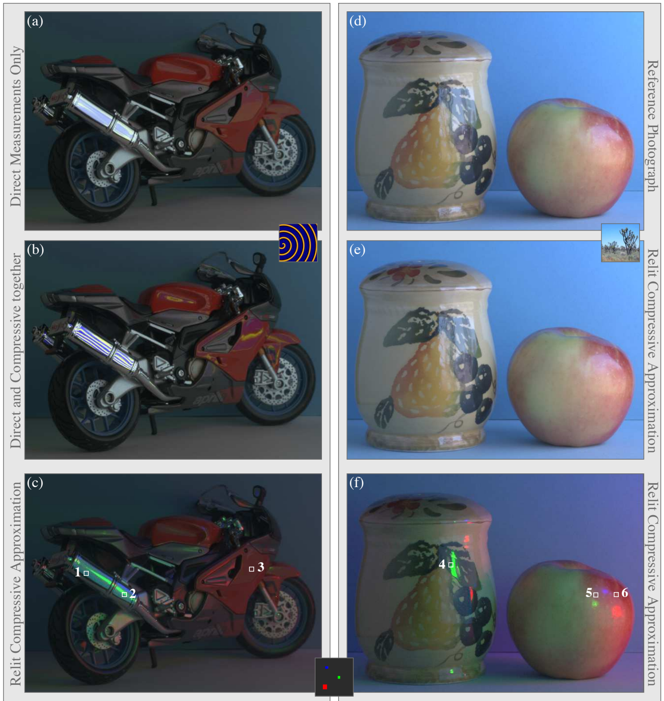
Figure 11: Acquired Reflectance Fields. Left column, a relit toy motorbike is shown. (a) and (b) are lit by the illumination condition shown in the inset. Subfigure (a) only shows the effect of directly measured coefficients, while (b) also includes the coefficients obtained by compressive sensing. (c) shows the motorbike relit by three colored light sources. The right column shows a ceramic object and an apple. A reference photograph of the scene (d) lit by the illumination condition (shown in the inset) is compared to a computed result (e). (f) shows the scene under three small colored light sources. Reflectance functions of the six marked pixels are shown in Figure 12.
