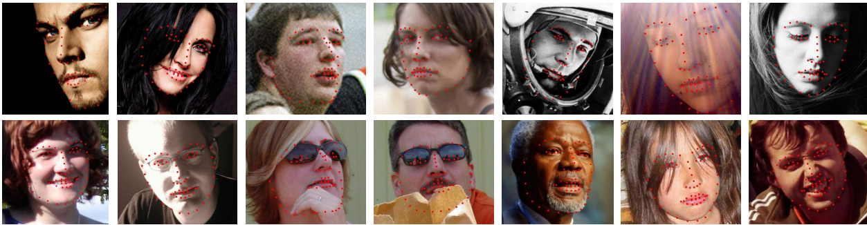
Figure 6: Examples of landmark detections in the wild using CLNF. Top row is from IBUG dataset, bottom row from AFW. Notice the generalisability across pose, illumination, and expression. The model can also deal with occlusions.
