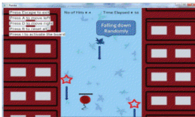
Figure 2. Screen shot of first prototype of the game. The player must navigate the balloon through a series of obstacles by shifting their weight on the balance board in the direction they want the balloon to move.
